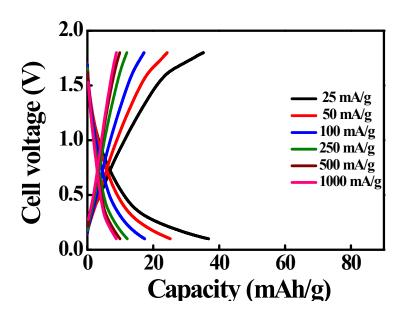
Figure S8. Charge–discharge curves of plain GNS electrode recorded in Li<sup>+</sup>-containing APC electrolyte with various current densities.
