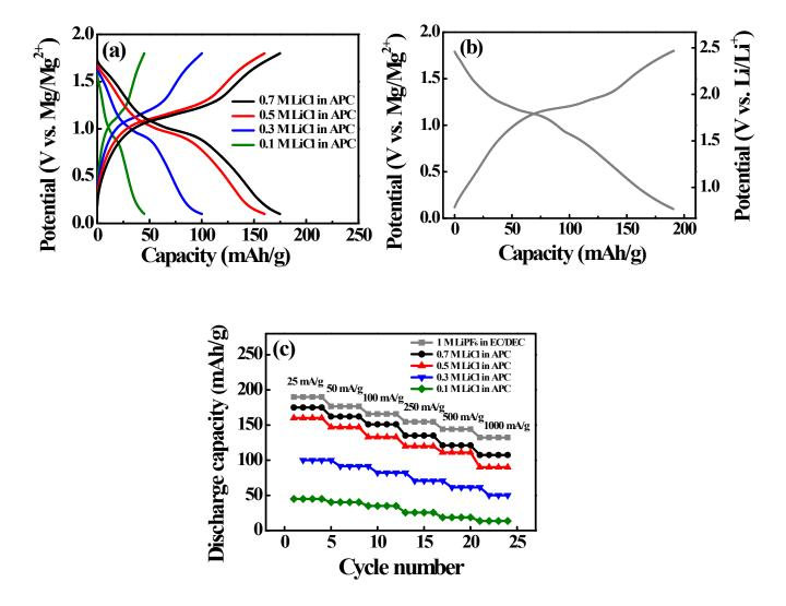
Figure S3. (a) Charge–discharge curves of MoS<sub>2</sub> electrode recorded in APC electrolytes with various LiCl concentrations. (b) Charge–discharge curves of MoS<sub>2</sub> electrode recorded in 1 M LiPF<sub>6</sub>/ethylene carbonate–diethyl carbonate electrolyte (with a Li counter). (c) Rate capability of MoS<sub>2</sub> electrode in various electrolytes.
