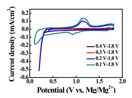
Figure S1. CV curves of  $MoS_2$  electrode recorded in Li<sup>+</sup>-containing APC electrolyte. Potential was scanned from 1.8 V to various lower limits with sweep rate of 0.1 mV/s. Results indicate that  $2H-MoS_2$  (before phase transformation at  $\sim$ 0.2 V) was inactive in this electrolyte.
