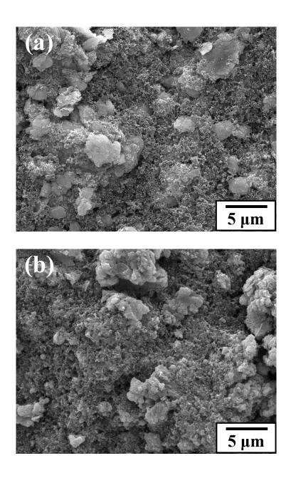
Figure S9. SEM micrographs of  $MoS_2$ -GNS electrode before and after being tested in  $Li^+$ -containing APC electrolyte for 200 charge—discharge cycles.
