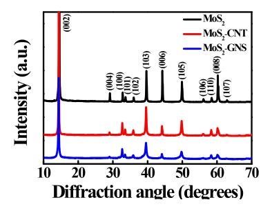
Figure S5. XRD patterns of as-received MoS<sub>2</sub>, MoS<sub>2</sub>-CNT, and MoS<sub>2</sub>-GNS samples.
