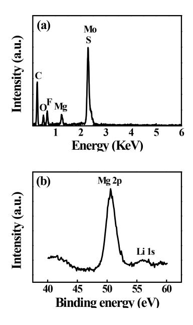
Figure S2. (a) EDS and (b) XPS analyses of  $MoS_2$  electrode after being discharged to 0.1 V.
