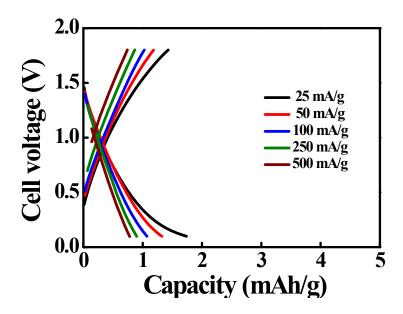
Figure S4. Charge–discharge curves of fresh  $MoS_2$  electrode recorded in plain APC electrolyte (without  $Li^+$ ).
