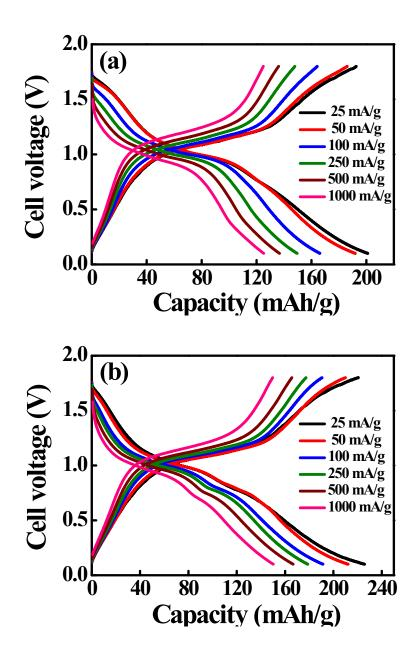
Figure S7. Charge–discharge curves of (a) MoS<sub>2</sub>-CNT and (b) MoS<sub>2</sub>-GNS electrodes recorded in Li<sup>+</sup>-containing APC electrolyte with various current densities.
