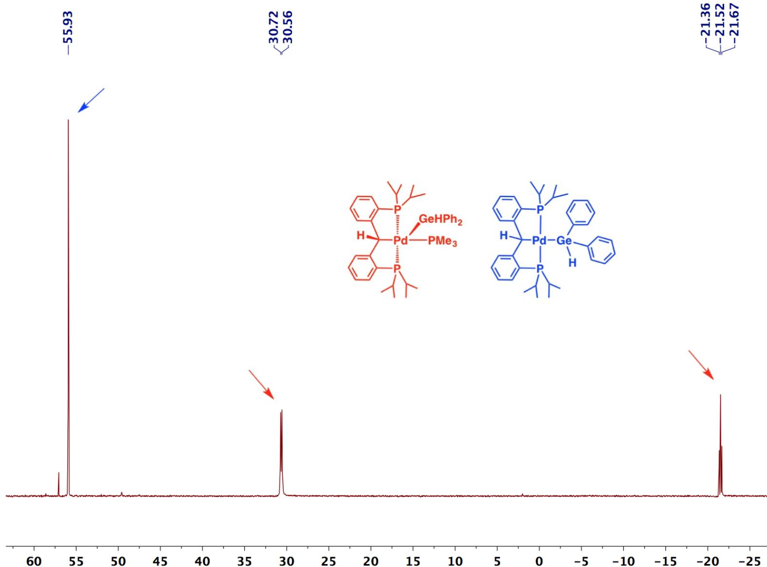
**Figure S54.**  $^{31}\text{P}\{\text{H}\}$  NMR spectrum for the mixture of  $[\text{PC}(\text{H})\text{P}] \text{Pd}(\text{PMe}_3)(\text{GeHPh}_2)$  (**13**) and  $[\text{PC}(\text{H})\text{P}] \text{Pd}(\text{GeHPh}_2)$  (**11**).
