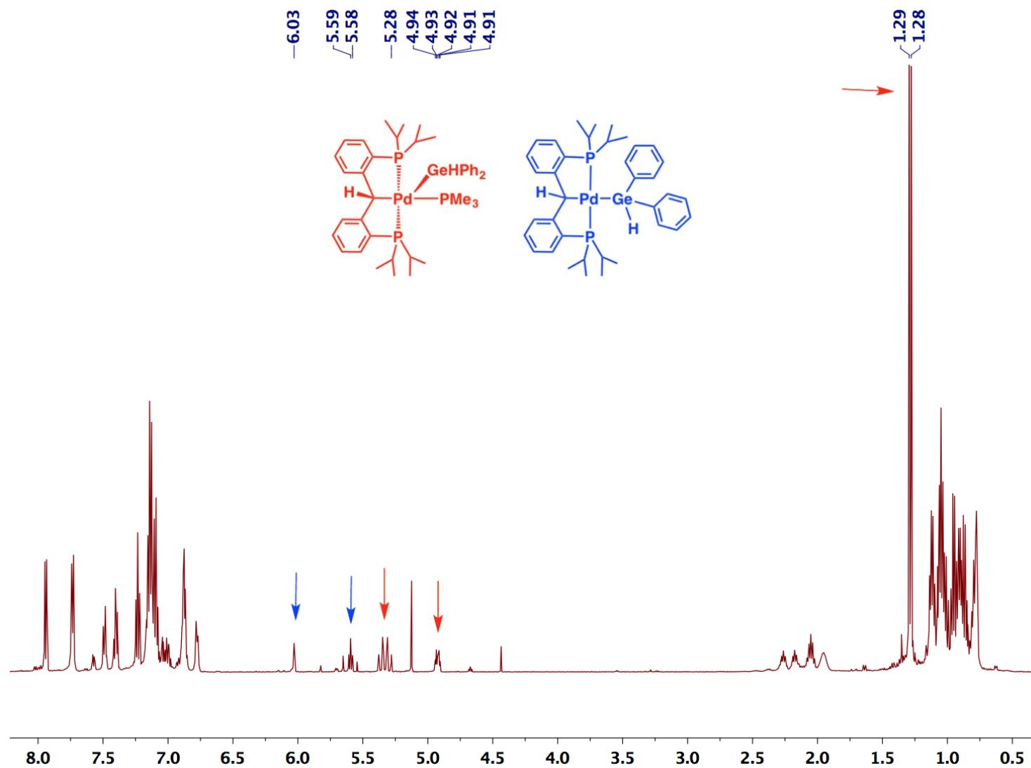
**Figure S53.**  $^1\text{H}$  NMR spectrum for the mixture of  $[\text{PC}(\text{H})\text{P}]\text{Pd}(\text{PMe}_3)(\text{GeHPh}_2)$  (13) and  $[\text{PC}(\text{H})\text{P}]\text{Pd}(\text{GeHPh}_2)$  (11).
