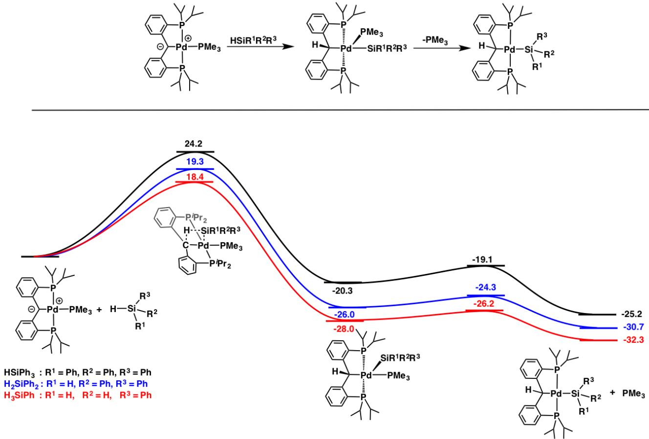
**Figure S3.** Calculated mechanism and reaction profile for the formation of the silyl products from  $[PC(sp^2)P]Pd(PMe_3)$  (1).
