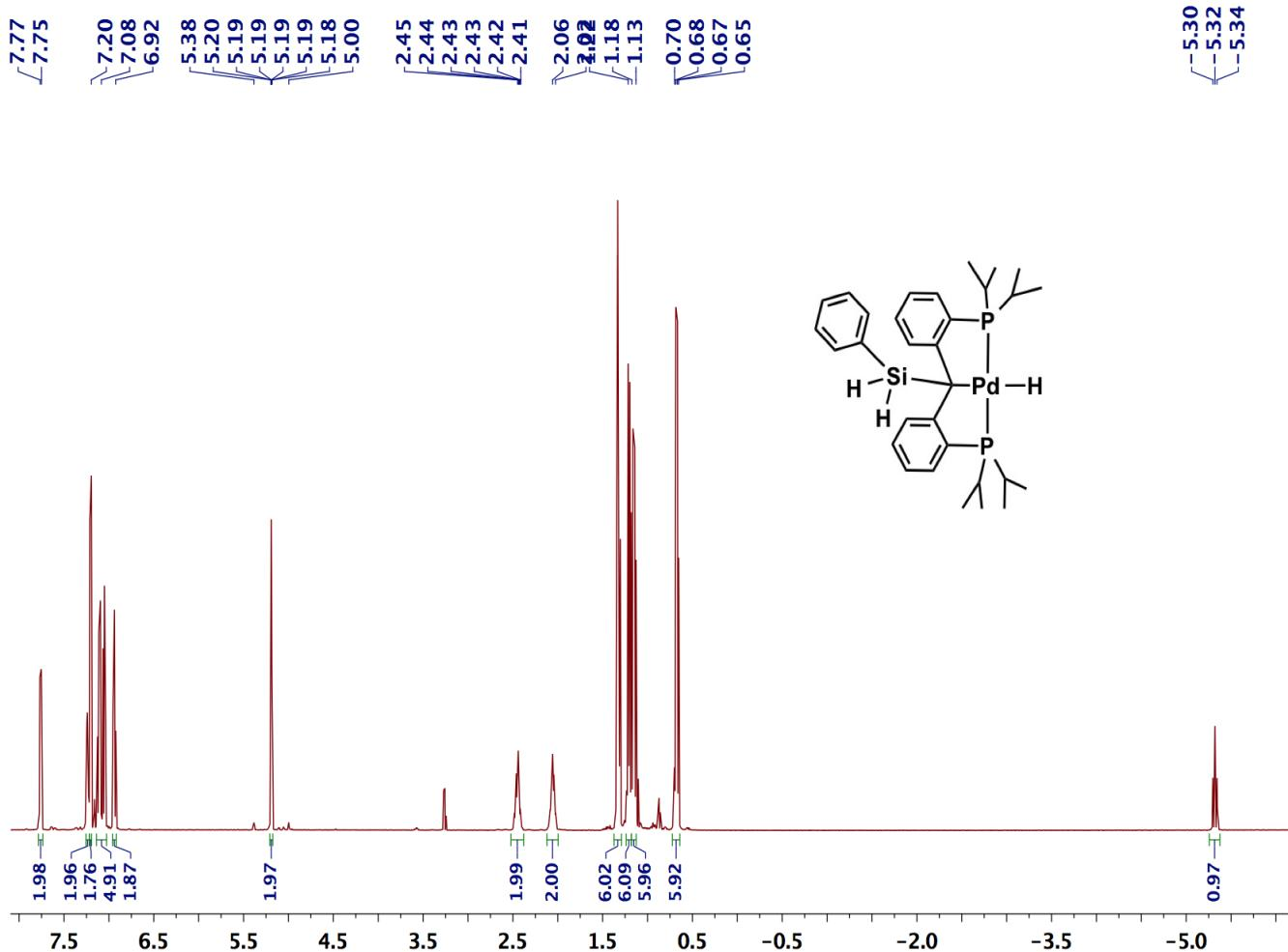
**Figure S7.** <sup>1</sup>H NMR spectrum for [PC(SiH<sub>2</sub>Ph)P]PdH (3).
