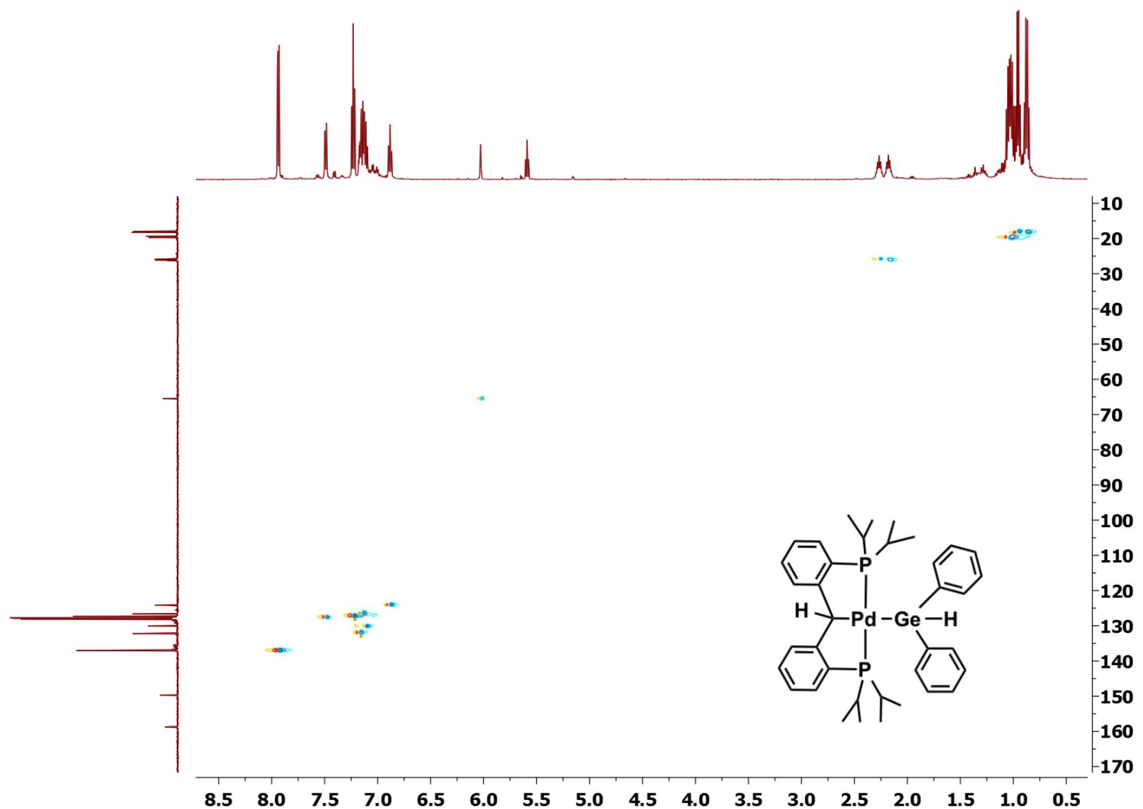
**Figure S46.**  $^1\text{H}$ - $^{13}\text{C}$  HSQC NMR spectrum for  $[\text{PC}(\text{H})\text{P}] \text{Pd}(\text{GeHPh}_2)$  (**11**).
