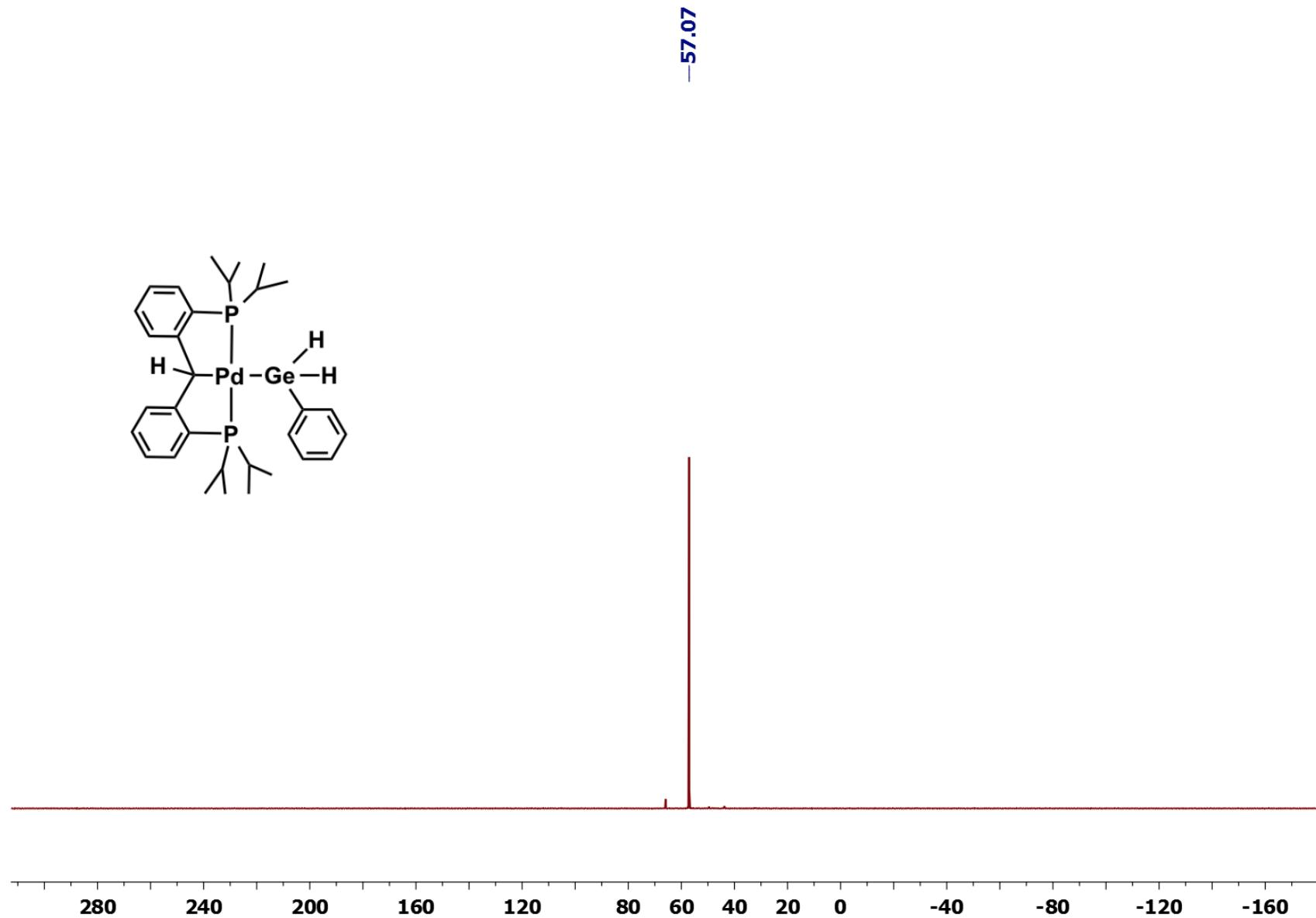
**Figure S39.**  $^{31}\text{P}\{\text{H}\}$  NMR spectrum for  $[\text{PC}(\text{H})\text{P}] \text{Pd}(\text{GeH}_2\text{Ph})$  (**10**).
