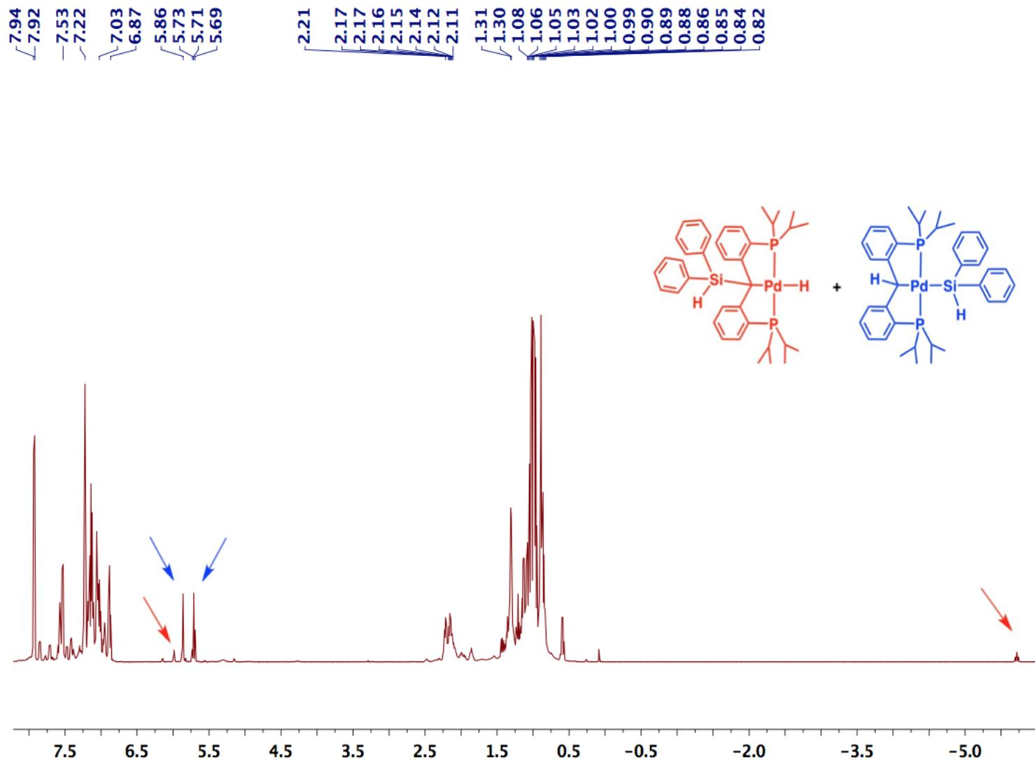
**Figure S22.** <sup>1</sup>H NMR spectrum for the mixture of [PC(H)P]Pd(SiHPh<sub>2</sub>) (7) and [PC(SiHPh<sub>2</sub>)P]PdH (4).
