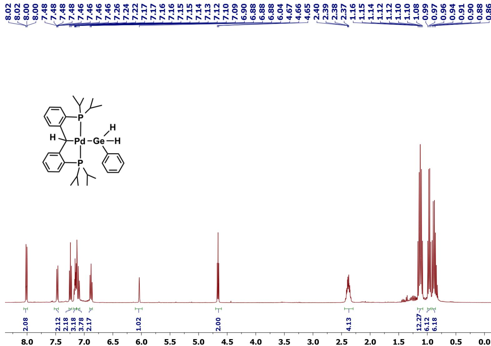
**Figure S38.**  $^1\text{H}$  NMR spectrum for  $[\text{PC}(\text{H})\text{P}]\text{Pd}(\text{GeH}_2\text{Ph})$  (**10**).
