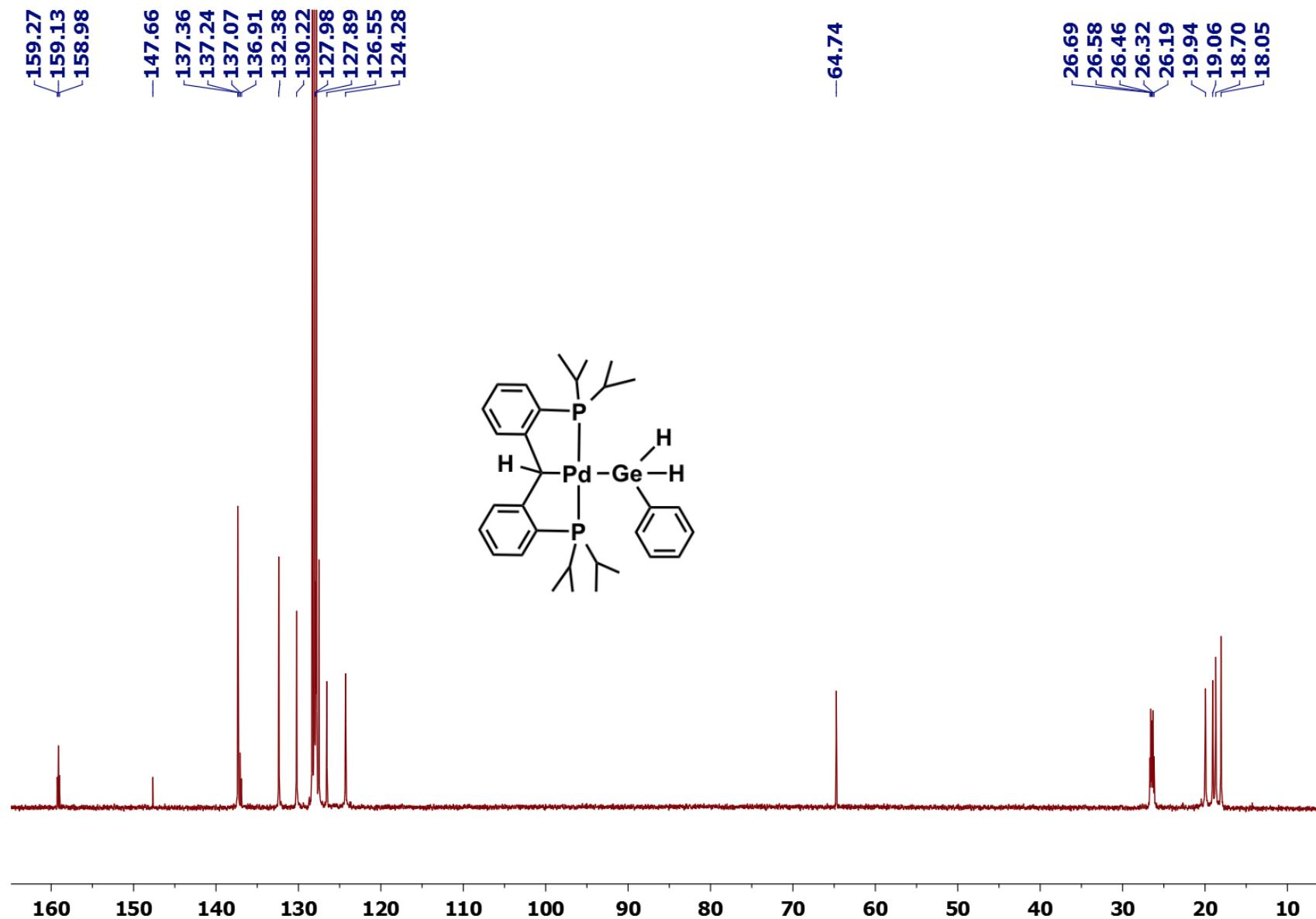
**Figure S40.**  $^{13}\text{C}\{^1\text{H}\}$  NMR spectrum for  $[\text{PC}(\text{H})\text{P}] \text{Pd}(\text{GeH}_2\text{Ph})$  (**10**).
