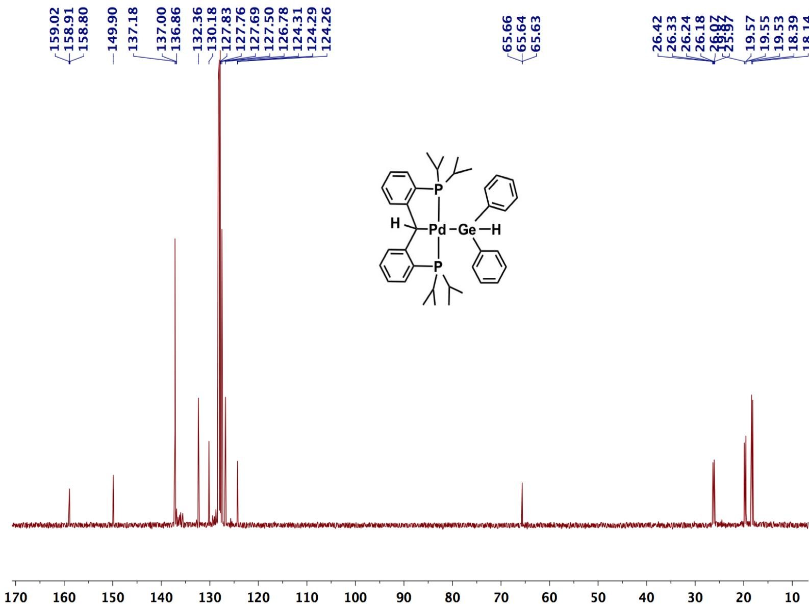
**Figure S45.**  $^{13}\text{C}\{^1\text{H}\}$  NMR spectrum for  $[\text{PC}(\text{H})\text{P}] \text{Pd}(\text{GeHPh}_2)$  (**11**).
