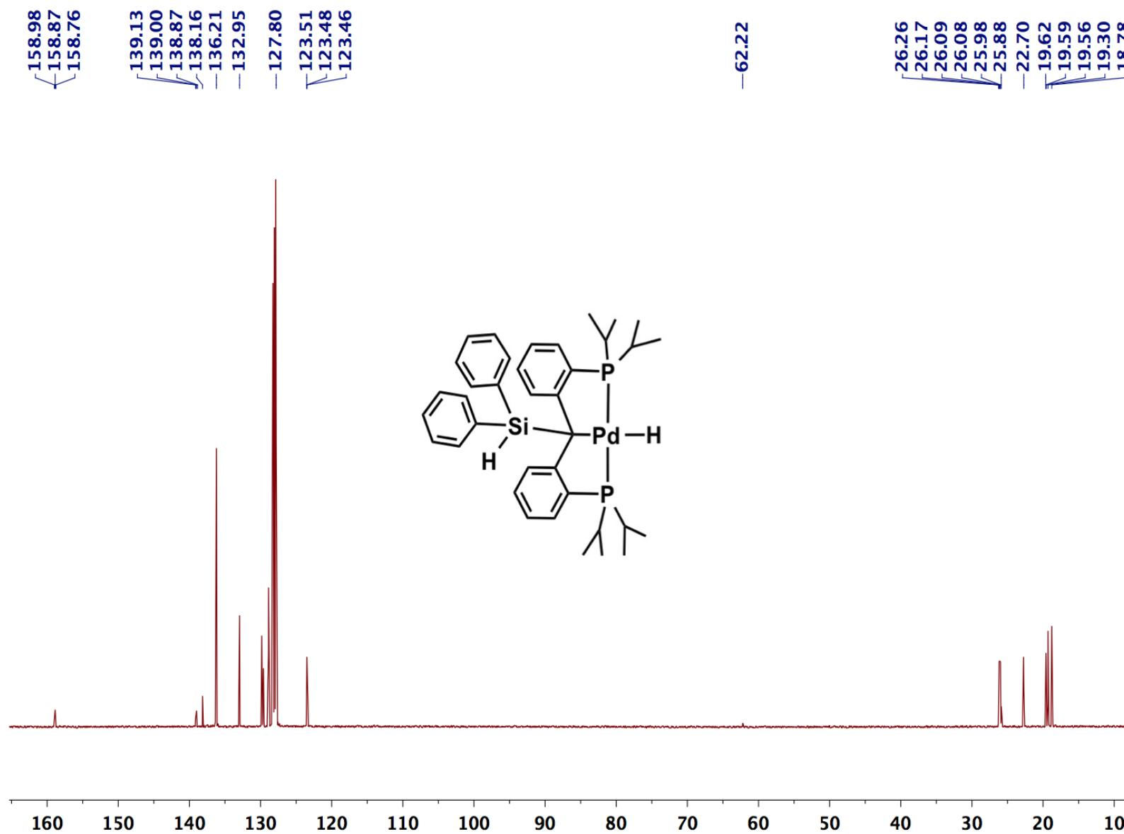
**Figure S14.**  $^{13}\text{C}\{^1\text{H}\}$  NMR spectrum for  $[\text{PC}(\text{SiHPh}_2)\text{P}] \text{PdH}$  (**4**).
