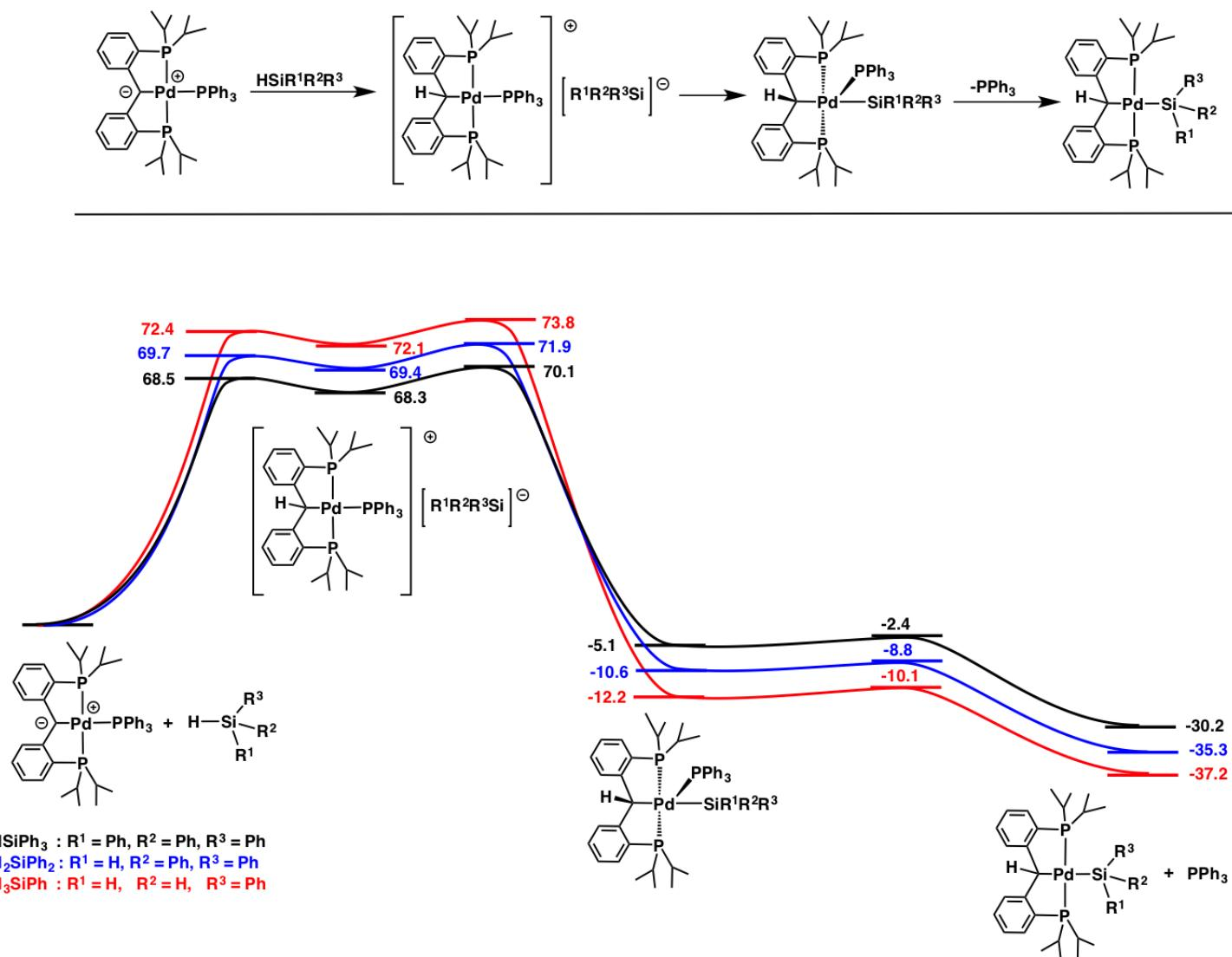
**Figure S6.** Calculated mechanism and reaction profile for the formation of the silyls from  $[PC(sp^2)P]Pd(PPh_3)$  (2) by a deprotonation mechanism.
