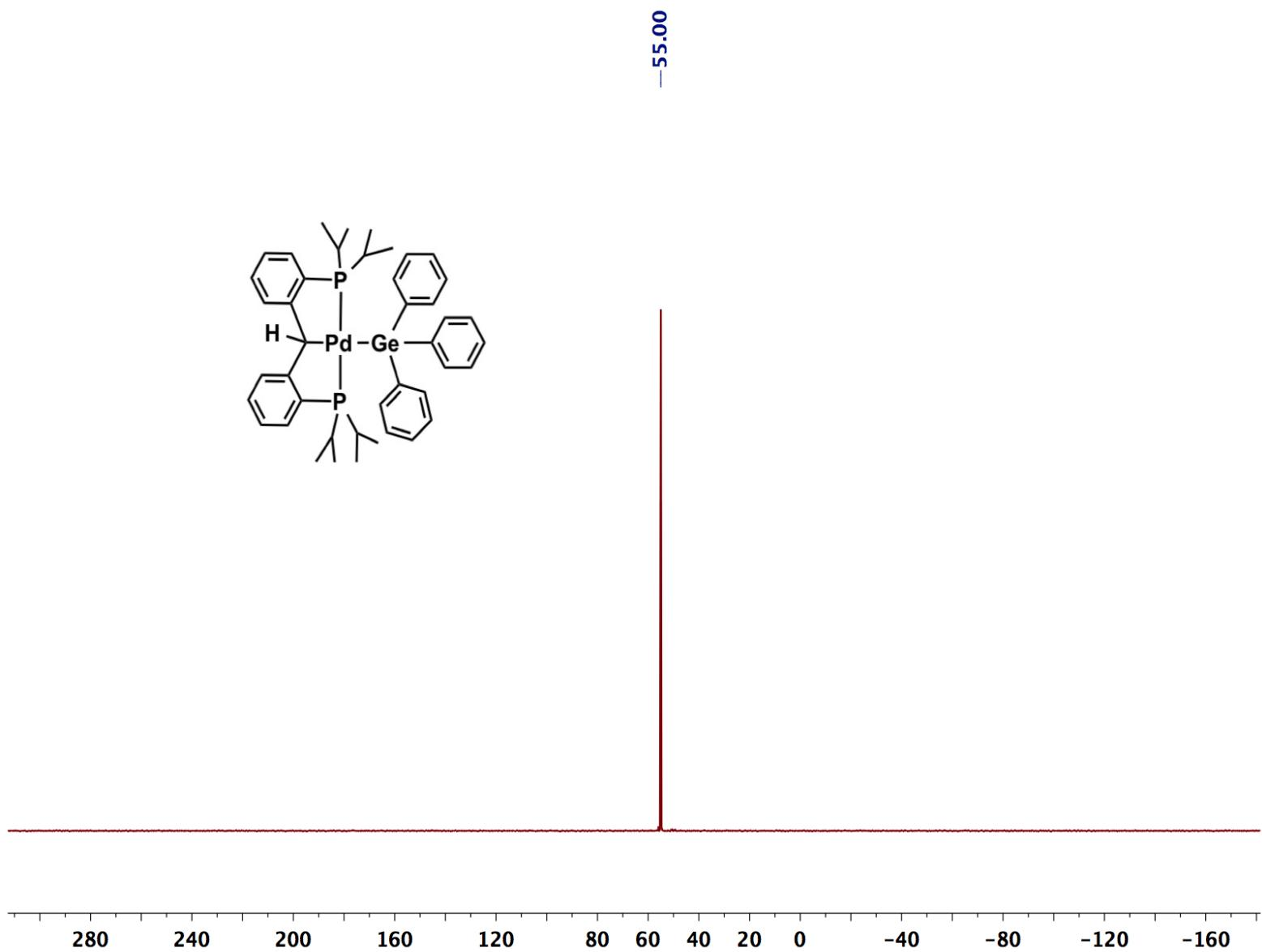
**Figure S48.**  ${}^{31}\text{P}\{{}^1\text{H}\}$  NMR spectrum for  $[\text{PC}(\text{H})\text{P}]\text{Pd}(\text{GePh}_3)$  (**12**).
