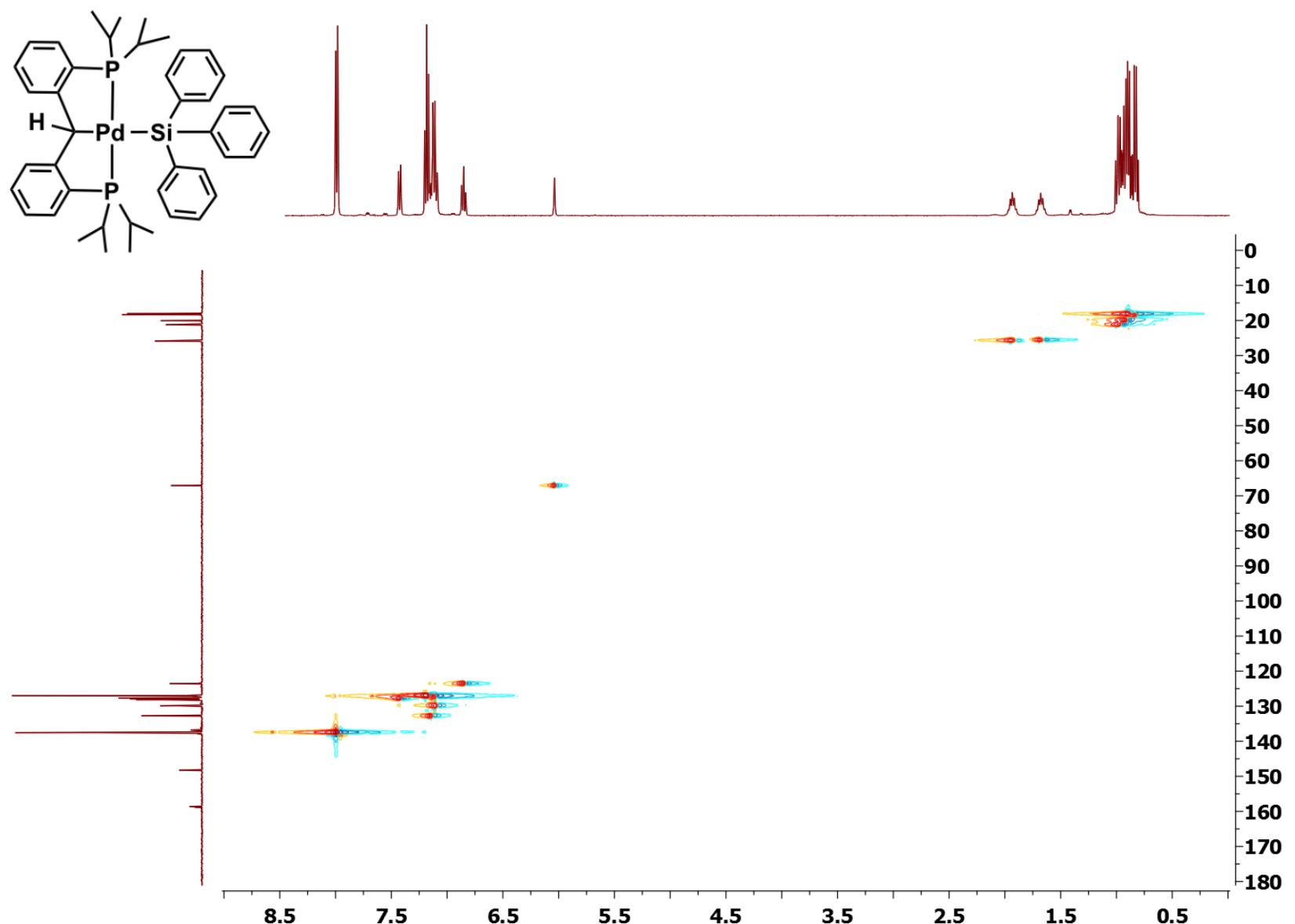
**Figure S30.**  $^1\text{H}$ - $^{13}\text{C}$  HSQC NMR spectrum for  $[\text{PC}(\text{H})\text{P}] \text{Pd}(\text{SiPh}_3)$  (8).
