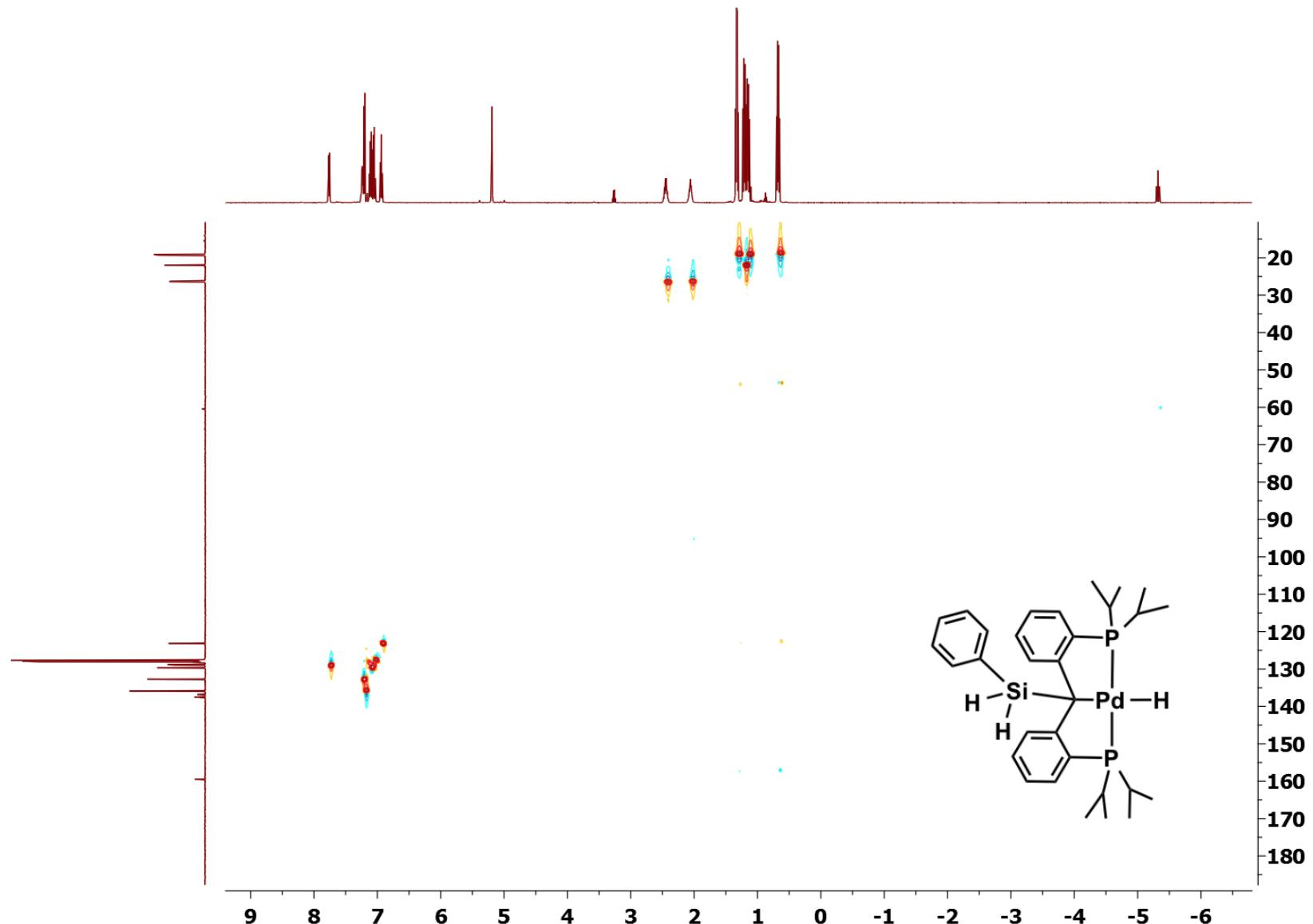
**Figure S11.**  $^1\text{H}$ - $^{13}\text{C}$  HSQC NMR spectrum for  $[\text{PC}(\text{SiH}_2\text{Ph})\text{P}]P\text{dH}$  (3).
