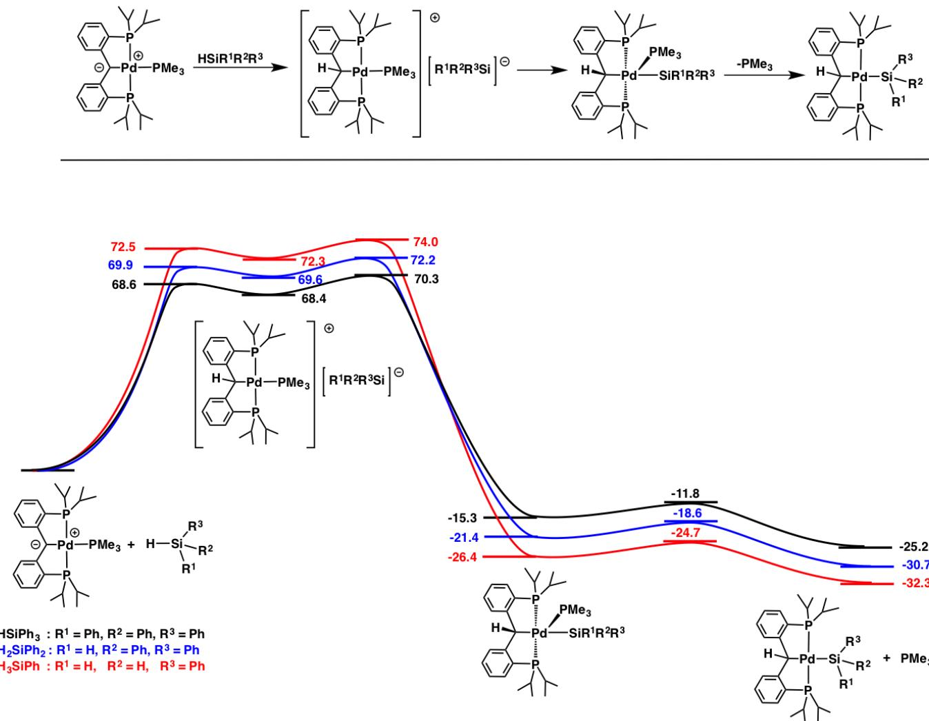
**Figure S5.** Calculated mechanism and reaction profile for the formation of the silyls from  $[PC(sp^2)P]Pd(PMe_3)$  (**1**) by a deprotonation mechanism.
