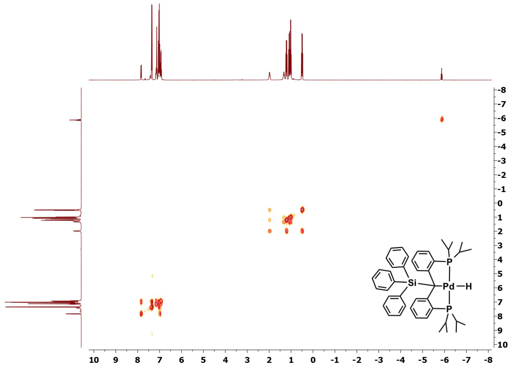
**Figure S21.**  $^1\text{H}$ - $^1\text{H}$  COSY NMR spectrum for  $[\text{PC}(\text{SiPh}_3)\text{P}] \text{PdH}$  (**5**).
