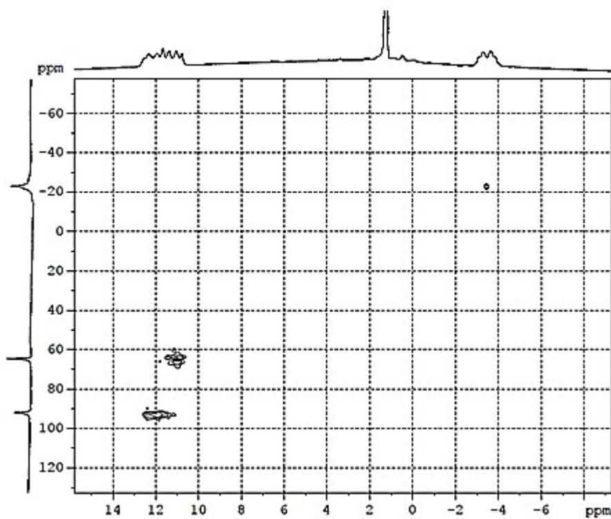
**Fig.S4.**  $^1\text{H}\{^{11}\text{B}\}$ - $^{11}\text{B}\{^1\text{H}\}$  HSQC spectrum of **1**
