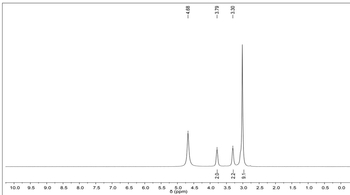
**Figure S14.**  $^1\text{H}$  NMR spectrum of choline chloride:zinc chloride ( $\text{CH}_3\text{OD}$ ) prepared by TSE.
