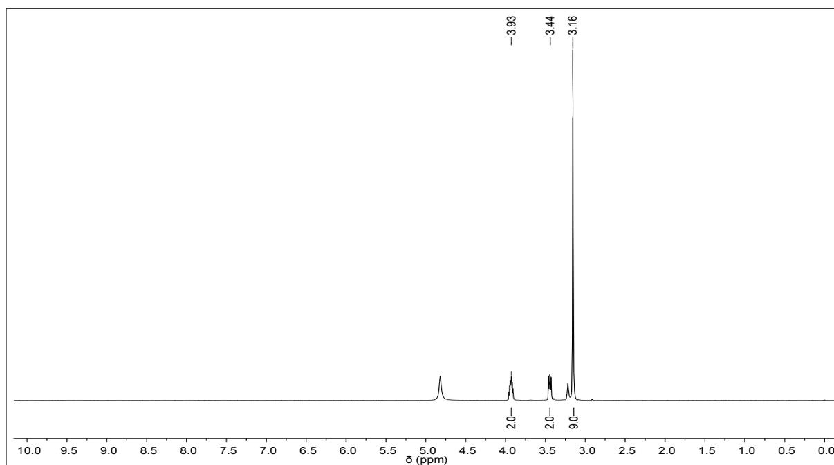
**Figure S13.**  $^1\text{H}$  NMR spectrum of choline chloride:zinc chloride ( $\text{CH}_3\text{OD}$ ) prepared by heating.
