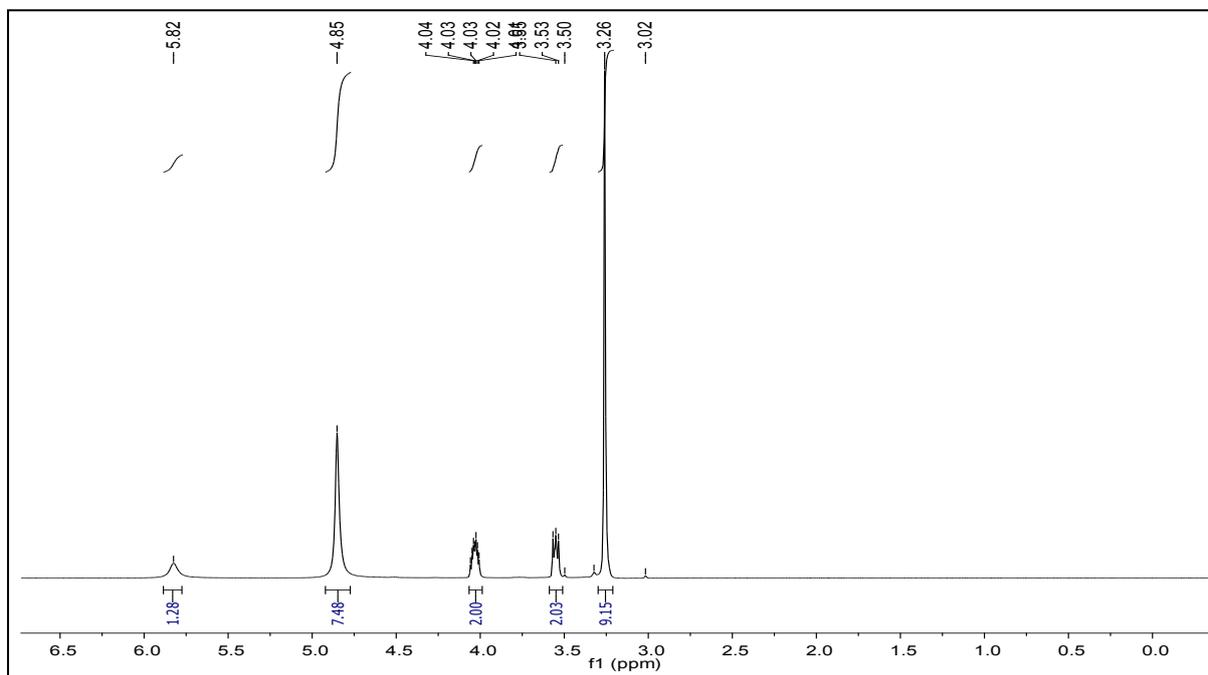
**Figure S1.**  $^1\text{H}$  NMR spectrum of Reline 200 ( $\text{CH}_3\text{OD}$ ) prepared by conventional heating.
