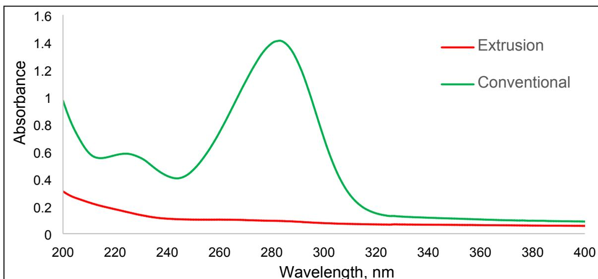
**Figure S12.** UV-Vis spectra of DES choline chloride: D-fructose made by TSE (red) and conventional heating (green).
