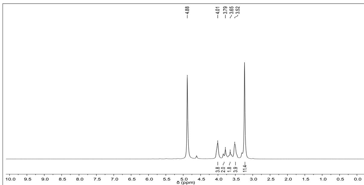
**Figure S10.**  $^1\text{H}$  NMR spectrum of choline chloride:D-fructose 200 ( $\text{CH}_3\text{OD}$ ) prepared by TSE.
