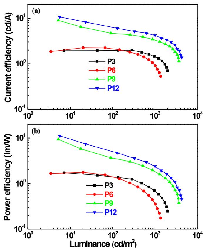
**Figure S6.** (a) Current efficiency versus luminance for the devices. (b) Power efficiency versus luminance for the devices.
