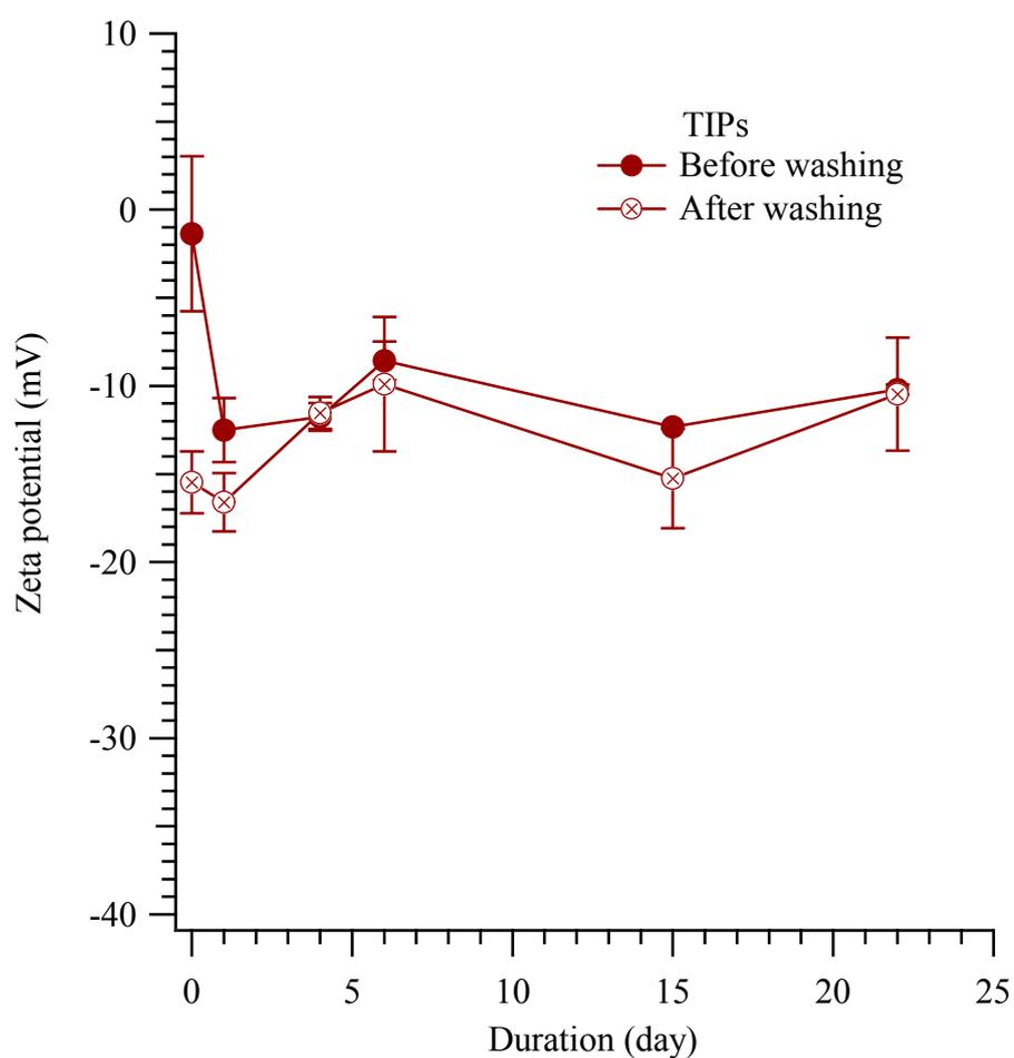
**Figure S2.** The Zeta potential of TIPs before and after template removal over three weeks.
