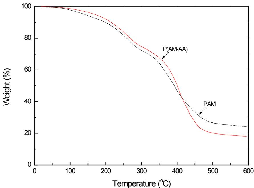
**Figure S6.** Thermogravimetric analyses of PAM and P(AM-AA) hydrogels.
