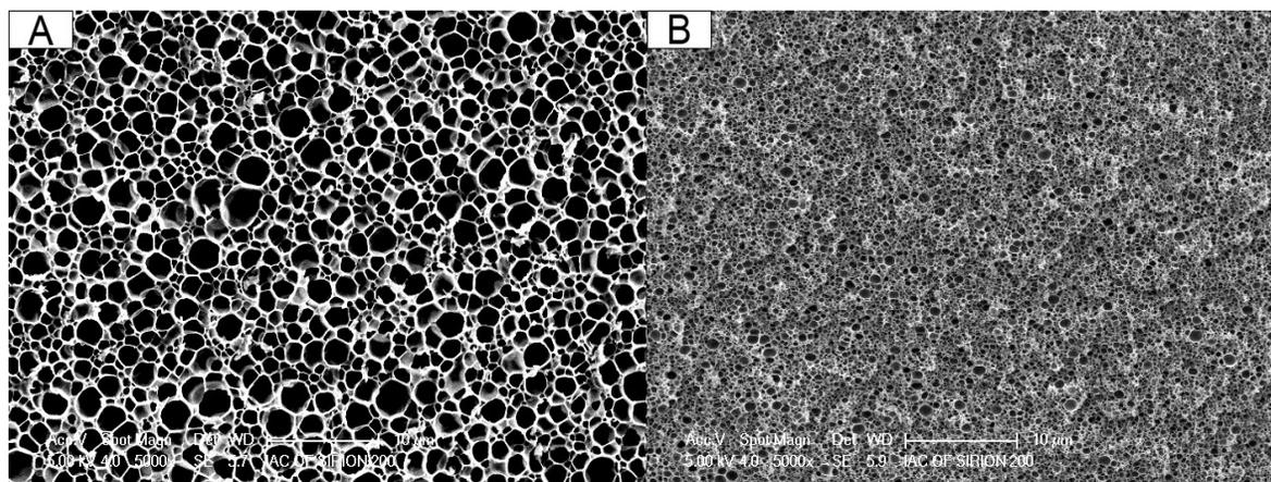
**Figure S4.** Whole SEM images of PAM gel (A) and P(AM-AA) gel (B).
