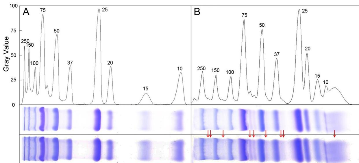
**Figure S3.** Comparative experiments of standard protein marker separation via P(AM-AA) gel under different running times of 90 minutes (A) and 100 minutes (B). The details of SDS-PAGE procedure was described in the supporting information given above. The red arrows indicate the minor protein bands separated via lengthened run of SDS-PAGE. The conditions were the same as those in Figure 2.
