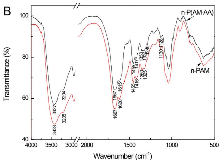
**Figure S5.** FTIR spectra of PAM and P(AM-AA) gels (A), n-PAM and n-P(AM-AA) gels (B).
