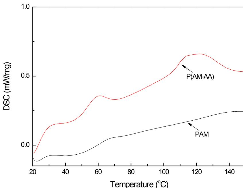
**Figure S7.** Thermogravimetric analyses (DSC) of PAM and P(AM-AA) hydrogels.
