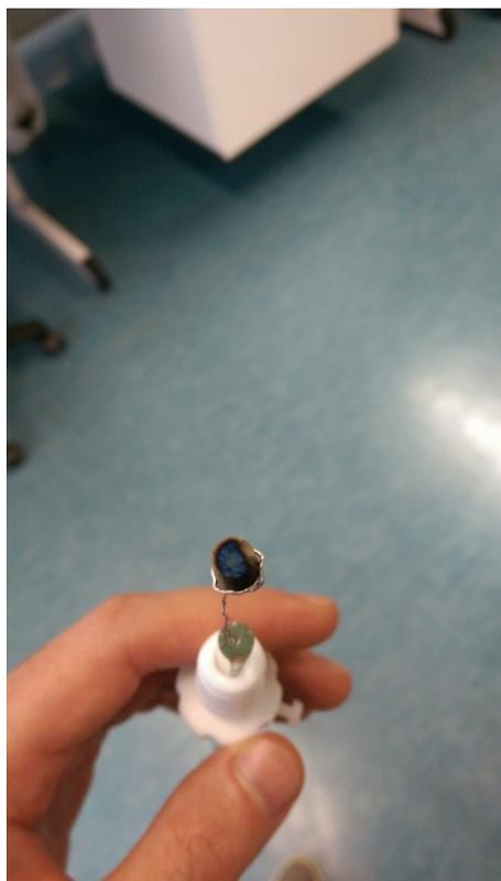
Fig. S15: Solid material deposited onto the PG electrode surface during OLEMS measurement of *trans*-[Fe(cyclam)Cl<sub>2</sub>] (**3**) in 0.1 M phosphate buffer (pH 7.5)
