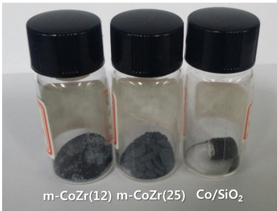
Figure S5. Photos of the used FTS catalysts after reaction, which showed a less aggregation of the catalyst particles due to the less wax deposition on the m-CoZr(12) and m-CoZr(25) compared to the conventional Co/SiO 2 having an irregular pore structures
