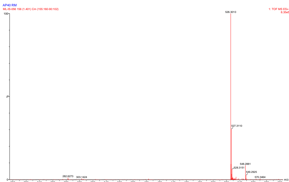
Figure S10: HRMS of compound 2 . Mass calcd for C_{23}H_{39}N_7O_7 : 525.2911, found M+H^+ = 526.3010 .
