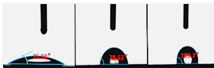
Figure S2. The contact angles of glass substrate, before- and after-calcined PVLs coating on glass slides.
