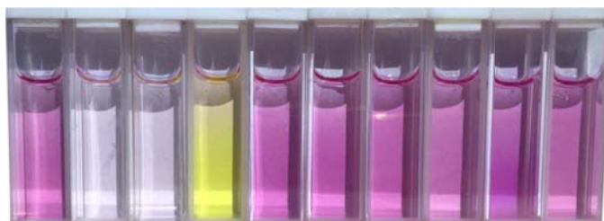
Figure S4. Image under visible light of CI-2 in PBS (pH 7.4, 10 mM) to various anions (Left to Right: probe (10 \mu\text{M} ), \text{Na}_2\text{SO}_3 (10 equiv.), \text{NaHSO}_3 (10 equiv.), \text{SO}_2 releasing agent (15 equiv. N-benzyl-2,4-dinitrobenzenesulfonamide and 150 equiv. Cys), \text{S}^{2-} (20 equiv.), Cys (1 mM), GSH (1 mM), Hcy (1 mM), donor (15 equiv.), other anions (1 mM)).
