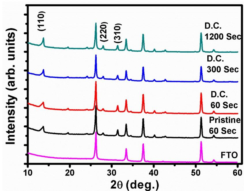
**S2: XRD of perovskite absorber layer annealed at 90°C for various post annealing time (60-1200 sec). (Pristine is single coating and DC refers to double coating)**
