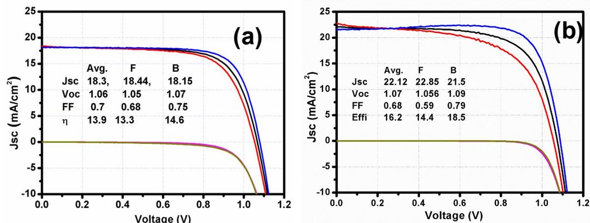
**S4: J-V curve of (a) single and (b) double coated perovskite devices.**
