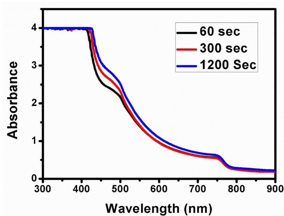
**S1: UV-Vis Spectrum of perovskite layer with various (60sec. to 1200 sec.) annealing times at 90 °C.**
