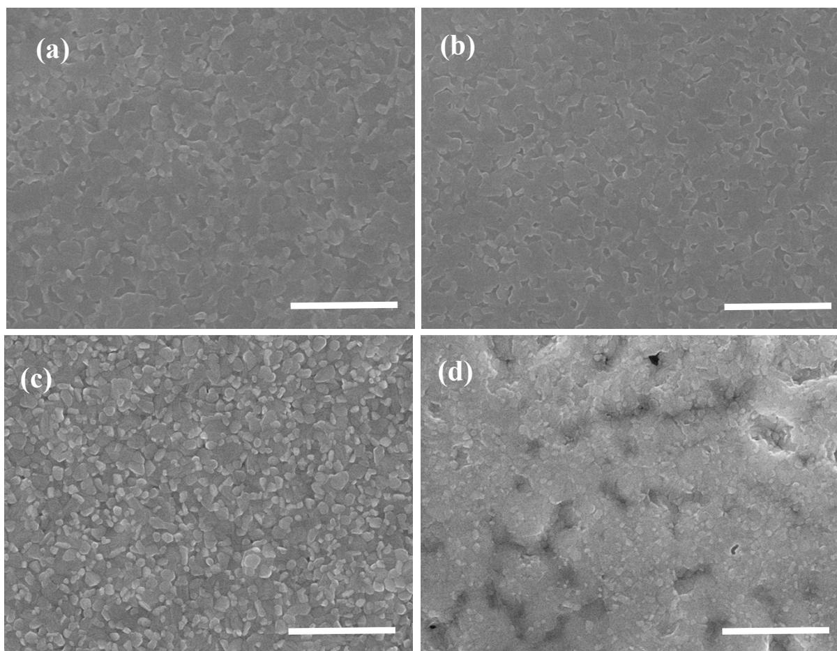
**S3. SEM top view of perovskite films with (a) Single coating. (b) double coating, (c) 3 cycle coating and (d) 5 cycle coating. The scale bar is 2 $\mu$ m.**
