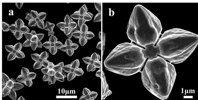
Figure S4. SEM images of 8-pods  $\text{Cu}_2\text{O}$ , (a) is the low magnification image, (b) is the high magnification image.
