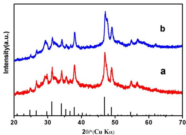
Figure S3. XRD patterns: a) 6-pods  $\text{Cu}_7\text{S}_4$  cages and b) type I 14-pods  $\text{Cu}_7\text{S}_4$  cages with PDF file No. 23-0598
