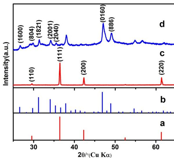
**Figure S1.** XRD patterns: a)  $\text{Cu}_2\text{O}$  with PDF file No. 05-0667, b)  $\text{Cu}_7\text{S}_4$  with PDF file No. 23-0598. Patterns c,d) are the corresponding XRD patterns of 14-pods  $\text{Cu}_2\text{O}$  and  $\text{Cu}_7\text{S}_4$  hollow cages, respectively.
