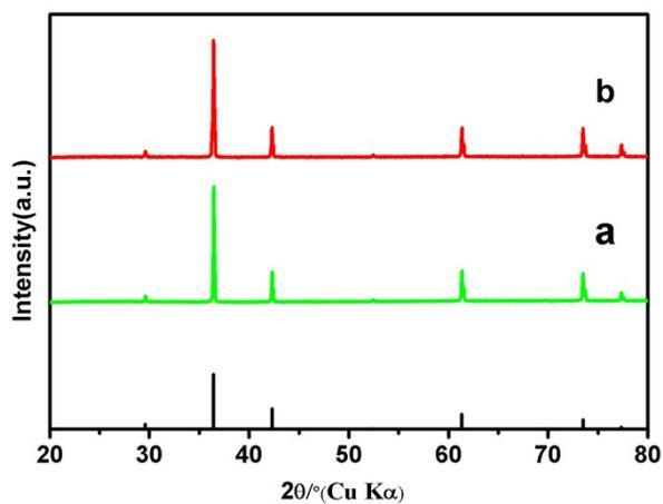
Figure S2. XRD patterns: a) 6-pods  $\text{Cu}_2\text{O}$  and b) type I 14-pods  $\text{Cu}_2\text{O}$  with PDF file No. 05-0667
