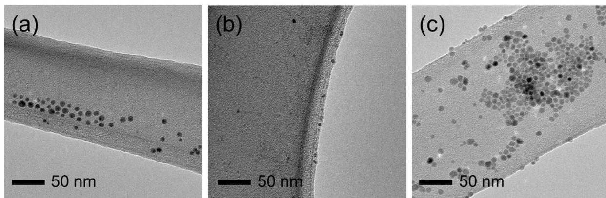
**Fig. S1** TEM images of (a) Ag@FeCo NPs which were sampled at 250 °C, (b) Co<sub>x</sub>Fe<sub>1-x</sub>O NPs which were sampled at 290 °C and (c) resulting Co<sub>x</sub>Fe<sub>1-x</sub>O NPs after the reaction.
