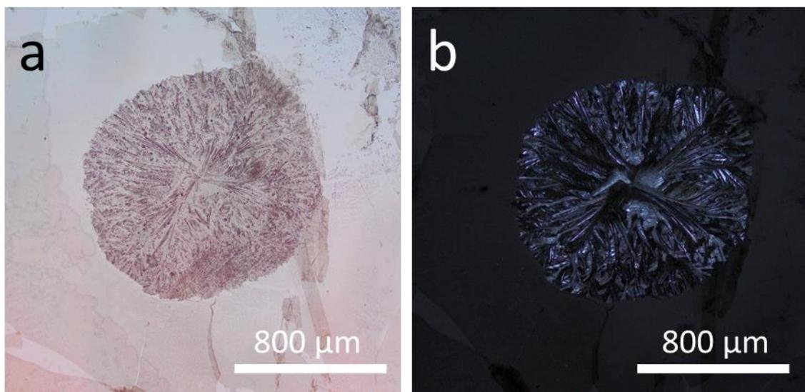
**Figure S2.** **a)** Optical micrograph of spherulite formed within an amorphous film at the air-water interface, removed from the reaction solution after 47 hours. **b)** Optical microscopy image of the same film taken with crossed polarizers at  $40^\circ$ , crystalline birefringent calcium carbonate spherulite evident within the non-birefringent amorphous film.
