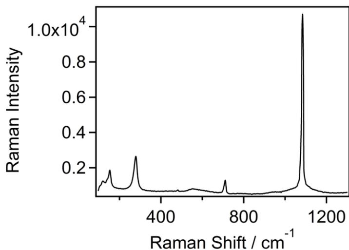
**Figure S7.** Raman spectra of calcium carbonate spherulites obtained after 96 hours of reaction time, Raman absorbance bands present ( $1085\text{ cm}^{-1}$ ,  $\nu_1$  symmetric stretch), ( $711\text{ cm}^{-1}$ ,  $\nu_4$  in-plane bending), ( $278$  and  $153\text{ cm}^{-1}$ , lattice modes) are concordant with calcite.
