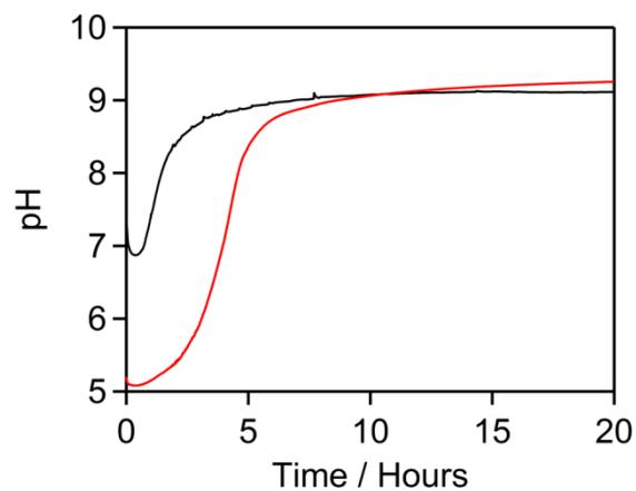
**Figure S15.** Reaction profile showing pH as a function of time for reaction solutions of differing initial pH. Black curve: starting pH of 7, red curve: starting pH of 5.
