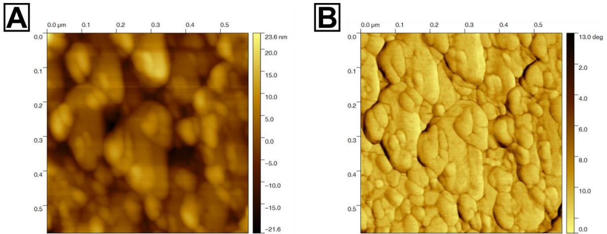
**Figure S14.** Standard AFM micrograph of the amorphous film obtained after 40 h. **A** height profile **B** phase image.
