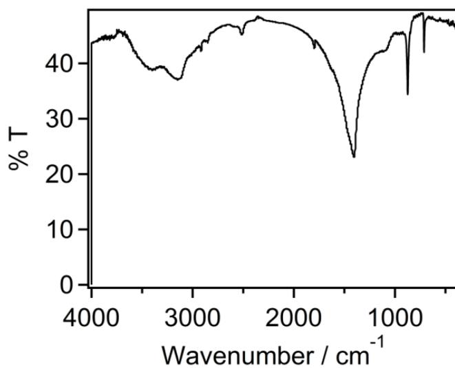
**Figure S8.** FTIR spectra of calcium carbonate spherulites removed from the reaction solution after 96 hours, absorbance bands present at  $1400$ ,  $872$  and  $712\text{ cm}^{-1}$  correspond to the  $\nu_3$ ,  $\nu_2$  and  $\nu_4\text{ CO}_3^{2-}$  bands of calcite respectively.
