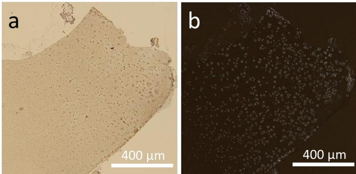
**Figure S1.** **a)** Optical micrograph of dried film formed at the air-water interface removed from the reaction solution after 40 hours. **b)** Optical microscopy image of the same film taken with crossed polarizers. Maltese crosses observed within the film indicate formation of crystalline birefringent calcium carbonate domains.
