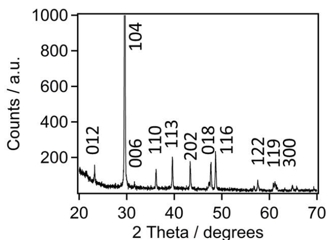
**Figure S6.** Powder XRD pattern of calcium carbonate spherulites removed from solution after a reaction time of 96 hours. Reflections at values of  $2\theta = 23, 29.5, 31.8, 36.1, 39.5, 43.2, 47.2, 47.6, 48.6, 56.6, 57.5, 60.7, 64.7$  and  $65.7^\circ$  correspond to the (012), (104), (006), (110), (113), (202), (024), (018), (116), (211), (122), (214), (300) and (0012) lattice planes of the calcium carbonate polymorph calcite respectively.
