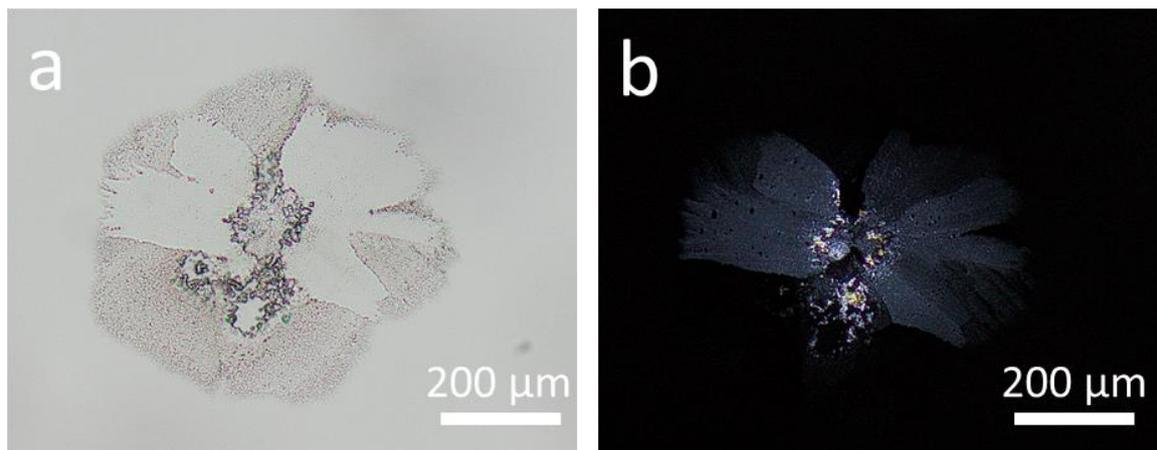
**Figure S3.** a) Optical micrograph of partially crystalline spherulite formed within an amorphous film at the air-water interface, removed from the reaction solution after 45 hours. b) Optical microscopy image of the same film taken with crossed polarizers, some domains within the calcium carbonate spherulite are crystalline as evidenced by birefringence, whereas other domains remain non-birefringent and amorphous.
