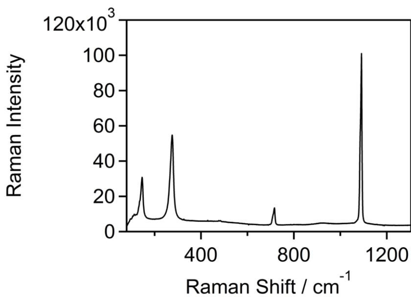
**Figure S4.** Raman spectra of calcium carbonate spherulites within amorphous film obtained after 52 hours of reaction time, Raman absorbance bands ( $1091\text{ cm}^{-1}$ ,  $\nu_1$  symmetric stretch), ( $716\text{ cm}^{-1}$ ,  $\nu_4$  in-plane bending), ( $276$  and  $146\text{ cm}^{-1}$ , lattice modes) are concordant with calcite.
