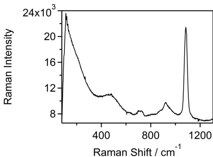
**Figure S5.** Raman spectra of amorphous calcium carbonate film obtained after 52 hours of reaction time, broad Raman absorbance bands present at 1082 and 712  $\text{cm}^{-1}$  correspond to the  $\nu_1$  and  $\nu_4$  modes of calcite respectively, the peaks at 112, 924 and 475  $\text{cm}^{-1}$  arise from PAA which is also present within the amorphous film.
