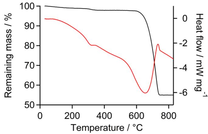
**Figure S13.** TGA (black line) and DSC (red line) profiles of calcium carbonate spherulites removed from solution after a reaction time of 96 hours.
