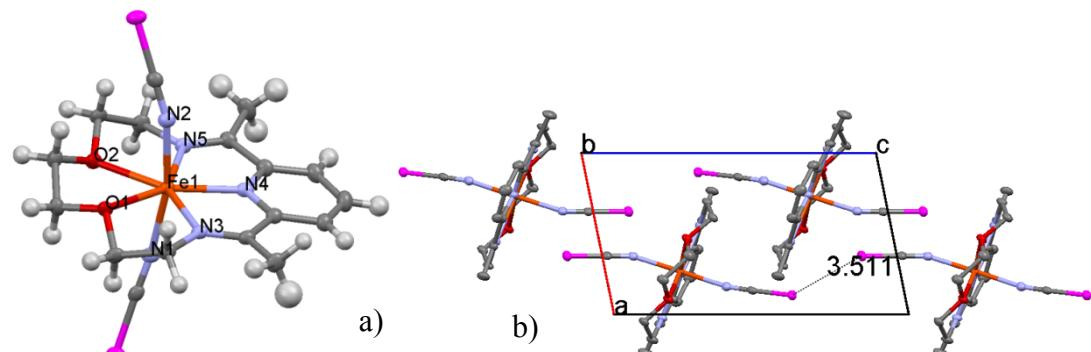
**Fig. S3** a) Molecular structure and b) Crystal packing of  $[\text{Fe}(\text{L}_{222}\text{N}_3\text{O}_2)(\text{NCSe})_2]$  at 100 K. Hydrogen atoms have been omitted for clarity in b.
