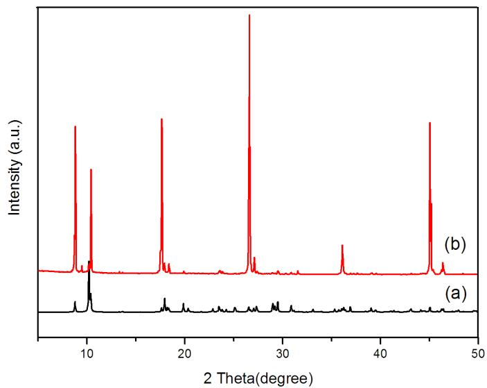
Fig. S4 The PXRD graph for complex 4 ((a) modulated by Mercury; (b) observed.)
