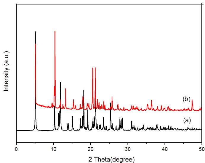
Fig. S5 The PXRD graph for complex 5 ((a) modulated by Mercury; (b) observed.)
