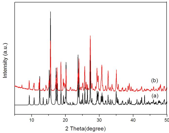
Fig. S1 The PXRD graph for complex **1** ((a) modulated by Mercury; (b) observed.)
