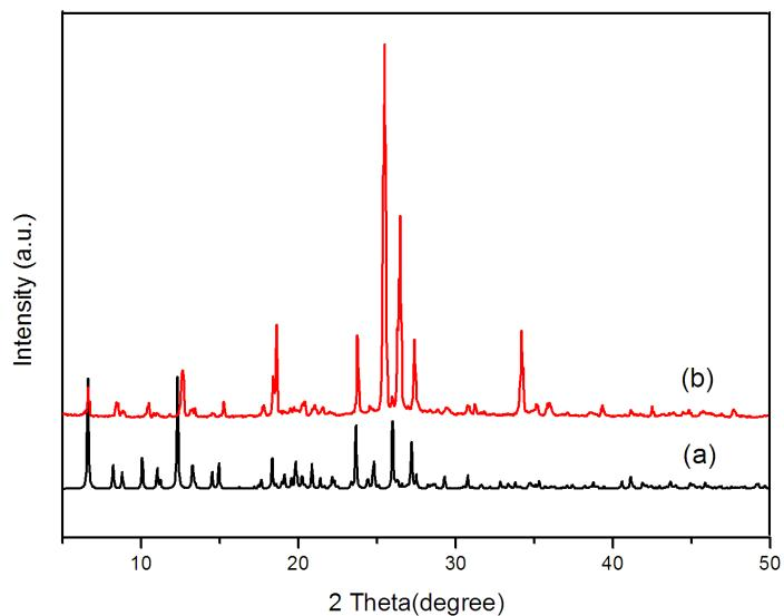
Fig. S7 The PXRD graph for complex **7** ((a) modulated by Mercury; (b) observed.)
