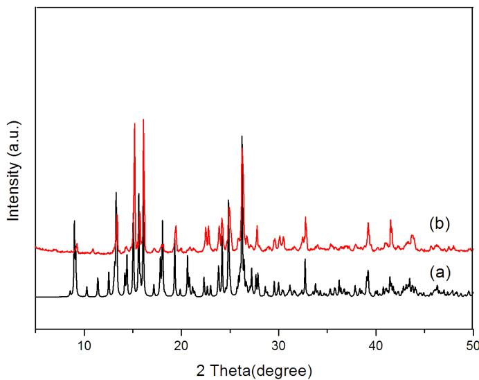
Fig. S6 The PXRD graph for complex 6 ((a) modulated by Mercury; (b) observed.)
