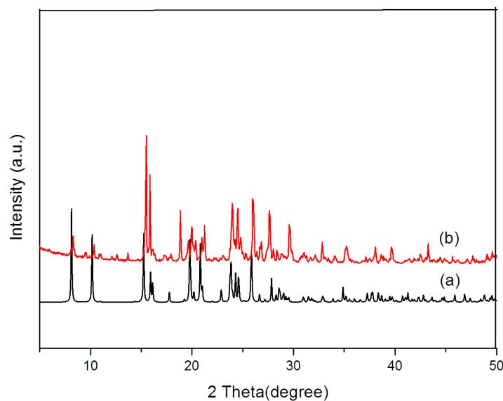
Fig. S2 The PXRD graph for complex **2** ((a) modulated by Mercury; (b) observed.)
