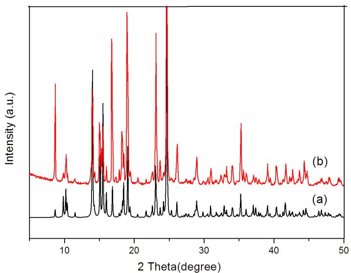
Fig. S3 The PXRD graph for complex 3 ((a) modulated by Mercury; (b) observed.)
