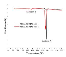
DSC profile of MRE (left). Thermal behaviour of 1:1 and 1:2 MRE:ACR crystal forms (right). Note the high temperature phase transition in metastable form II.
