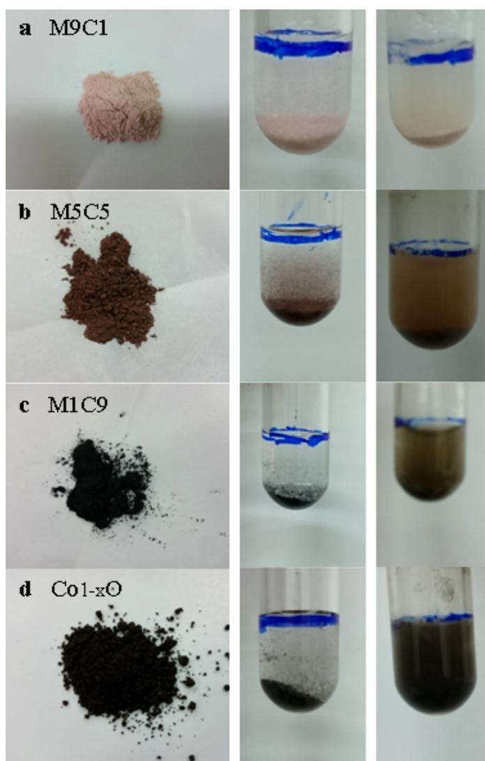
Supplement Figure 1. Photos of (a) M9C1, (b) M5C5 and (c) M1C9 solid solution powders (SSP) by reactive sintering at 1100°C for 3 h in air followed by grinding to be smaller than 100  $\mu\text{m}$  in size (left panel) and then dispersion in water (middle panel) for PLA in water for 5 min (right panel). For comparison, the Co<sub>1-x</sub>O powder of rocksalt-type structure (Aldrich, 325 mesh) was also subjected to PLA in water for 5 min as compiled in (d).
