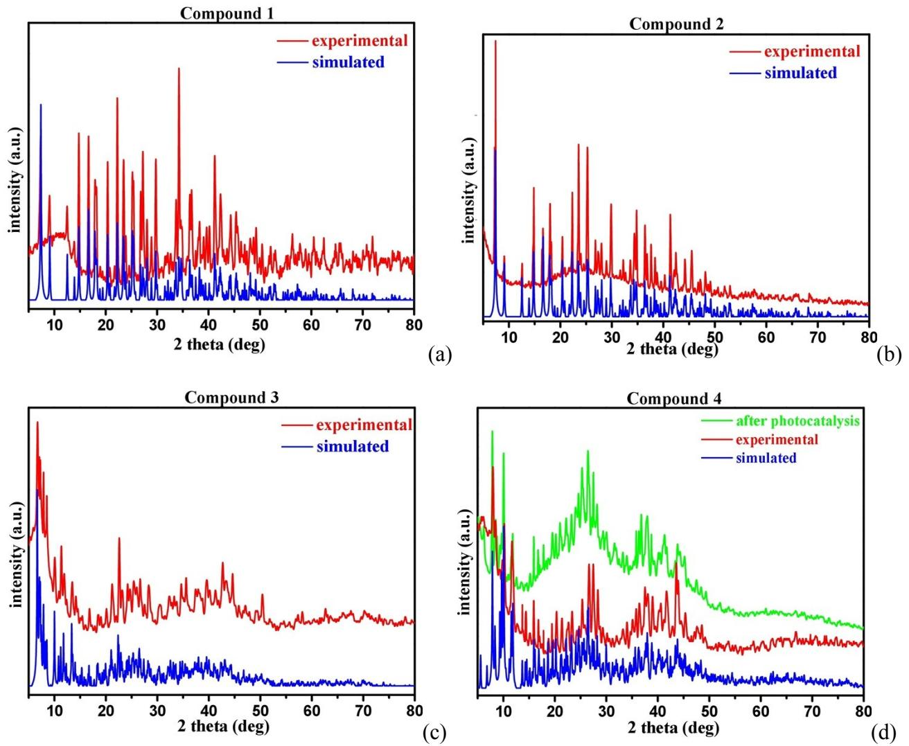
**Fig. S6** Experimental and simulated XRD powder patterns for compounds 1-4.
