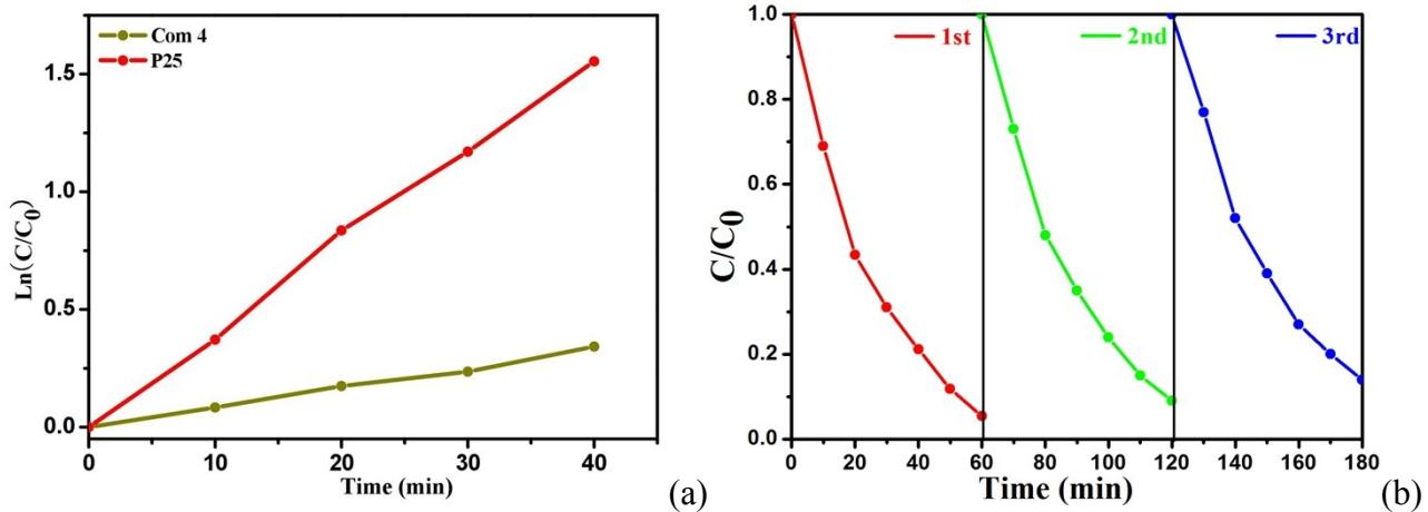
**Fig. S5** The linear relationship of  $\ln(C_0/C)$  over reaction time for RhB (a) and irradiation-time dependences of the relative concentration  $C/C_0$  of the RhB (b) dye over **4** during cycling photocatalytic experiments under visible light.
