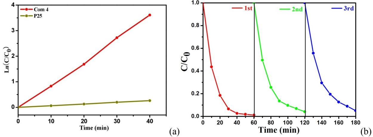
**Fig. S4** The linear relationship of  $\ln(C_0/C)$  over reaction time for CV (a) and irradiation-time dependences of the relative concentration  $C/C_0$  of the CV (b) dye over **4** during cycling photocatalytic experiments under visible light.
