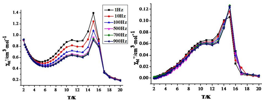
Figure S6 Temperature dependence of AC susceptibilities of **3** in  $H_{ac}=3$  Oe and  $H_{dc}=0$  Oe.
