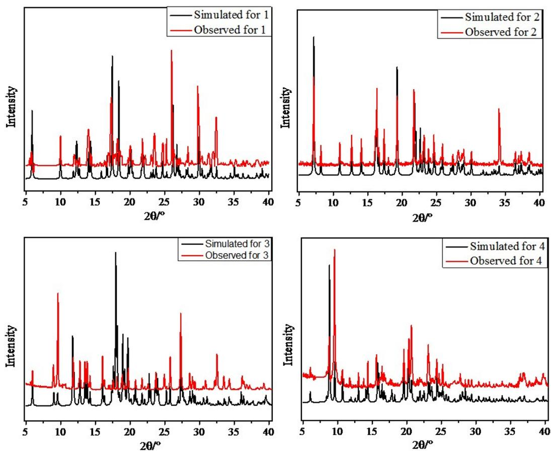
Figure S2. PXRD patterns of the series complexes. Black: Simulated from the X-ray single-crystal data; Red: observed for the as-synthesized solids.
