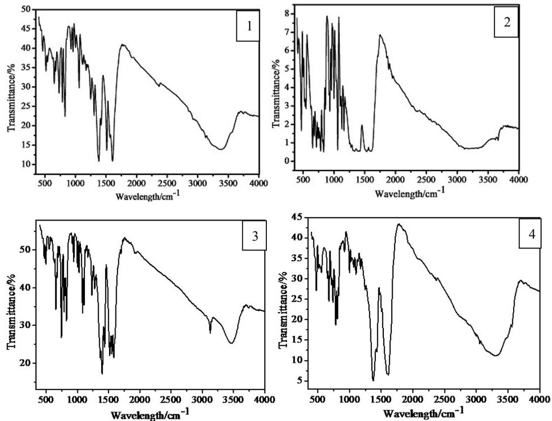
Figure S1. The IR spectra of the series complexes.
