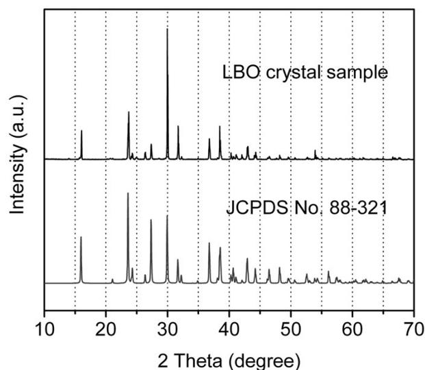
**Fig. S2** The XRD pattern of a LBO crystal sample used in our experiment (top) and the data in the JCPDS XRD standard card (JCPDS No. 88-321) for comparison (bottom).
