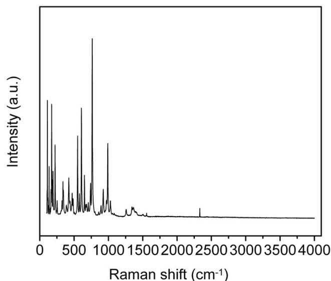
**Fig. S1** The Raman spectrum of a LBO crystal slice used in our experiments.
