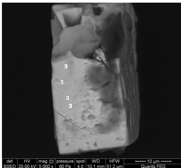
Figure S2(a) BSE image and EDS measuring points for \text{K}_2\text{MgTh}_3(\text{MoO}_4)_8
