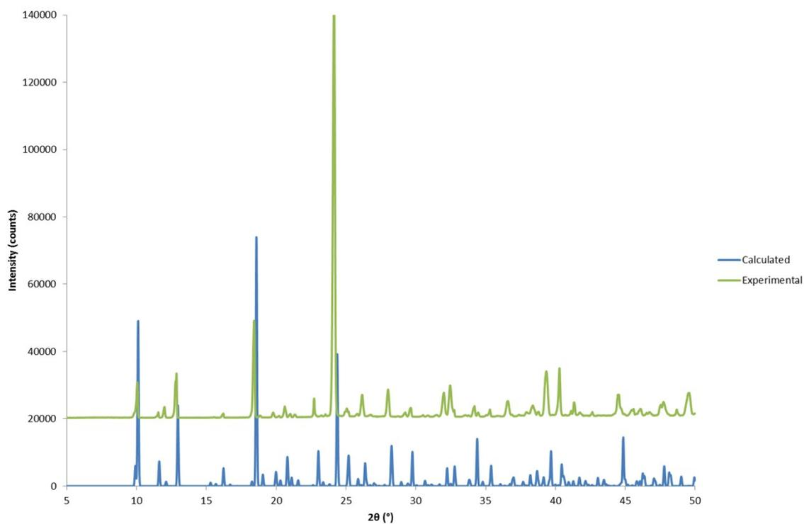
**Figure S1.1:** Calculated and experimental powder diffraction patterns for  $\text{Ni}_2(\text{mip})_2(\text{H}_2\text{O})_8 \cdot 2\text{H}_2\text{O}$  (1).
