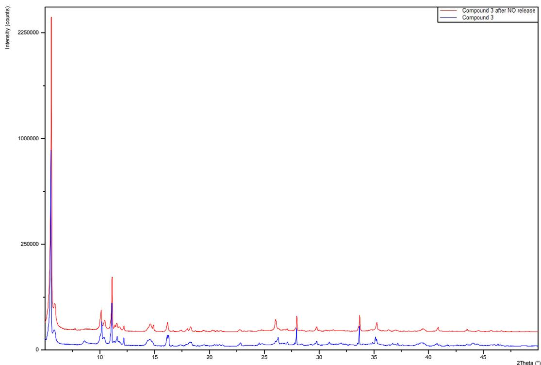
**Figure S4.2:** Comparison of PXRD patterns of Compound 3 as synthesised (blue) and after (red) dehydration and NO-loading and release experiments. The after NO release trace has been multiplied by a factor of 2.
