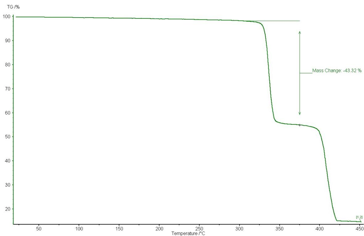
**Figure S2.4:** Thermogravimetric analysis of Compound **4**. The compound is stable up to approximately 300°C, at which point a mass loss occurs corresponding to more than the loss of both carboxylate groups (35.34%).
