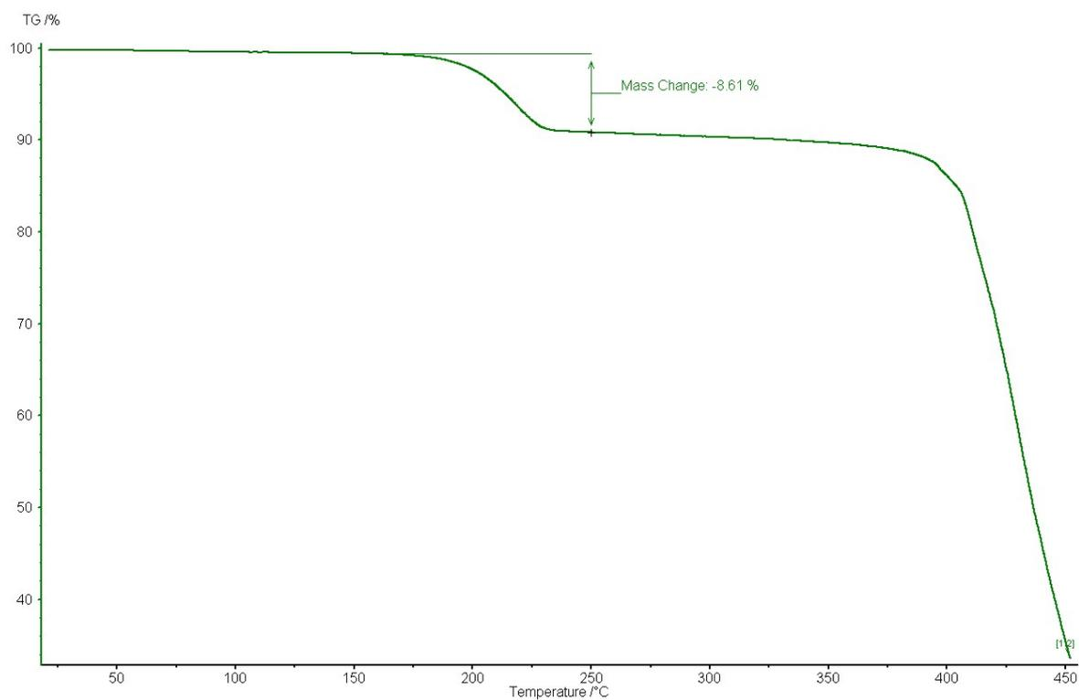
**Figure S2.5:** Thermogravimetric analysis of Compound **5**. The mass loss occurring over the 150° to 250°C temperature range approximately corresponds to the loss of the coordinated ethanol molecule (10.35%).
