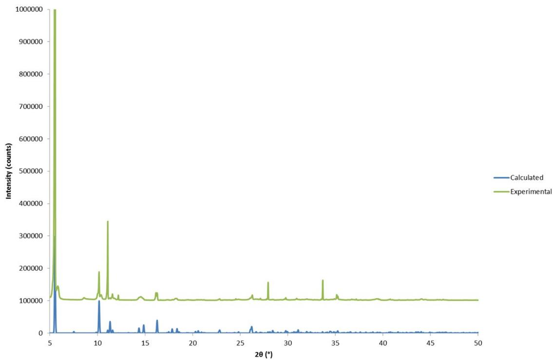
**Figure S1.3:** Calculated and experimental powder diffraction patterns for  $\text{Zn}_6(\text{mip})_5(\text{OH})_2(\text{H}_2\text{O})_2 \cdot 4\text{H}_2\text{O}$  (**3**).
