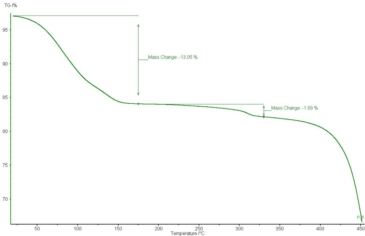
**Figure S2.2:** Thermogravimetric analysis of Compound 2. Initial mass loss occurring between 20 and 175°C corresponds to the loss of approximately 11 water molecules (13.07%).
