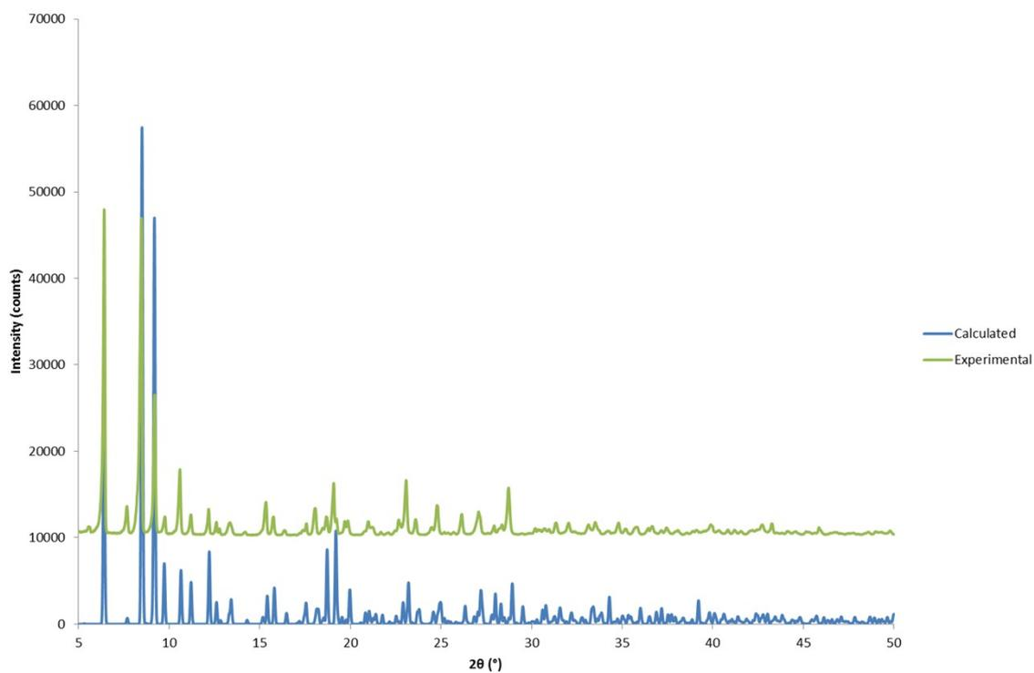
**Figure S1.2:** Calculated and experimental powder diffraction patterns for  $\text{Zn}_6(\text{mip})_5(\text{OH})_2(\text{H}_2\text{O})_4 \cdot 6.1\text{H}_2\text{O}$  (2).
