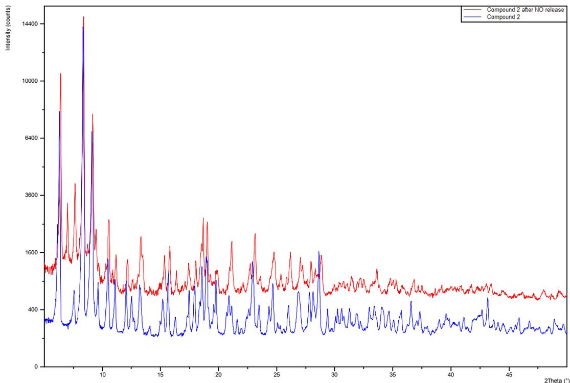
**Figure S4.1:** Comparison of PXRD patterns of Compound 2 as synthesised (blue) and after (red) dehydration and NO-loading and release experiments. The intensities of the as synthesised powder have been scaled down to 0.3 times their original intensity to for a clear comparison of the patterns.
