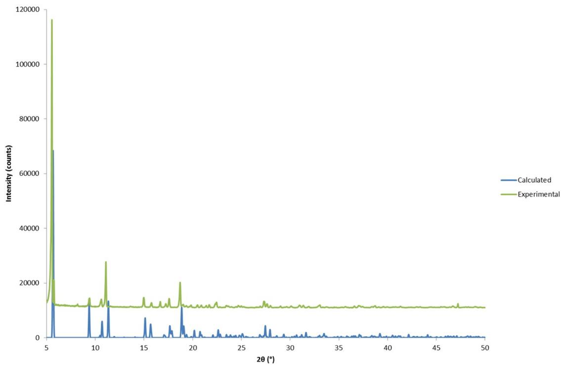
**Figure S1.5:** Calculated and experimental powder diffraction patterns for  $\text{Mn}_3(\text{tbip})_2(\text{Htbip})_2(\text{EtOH})_2$  (**5**).
