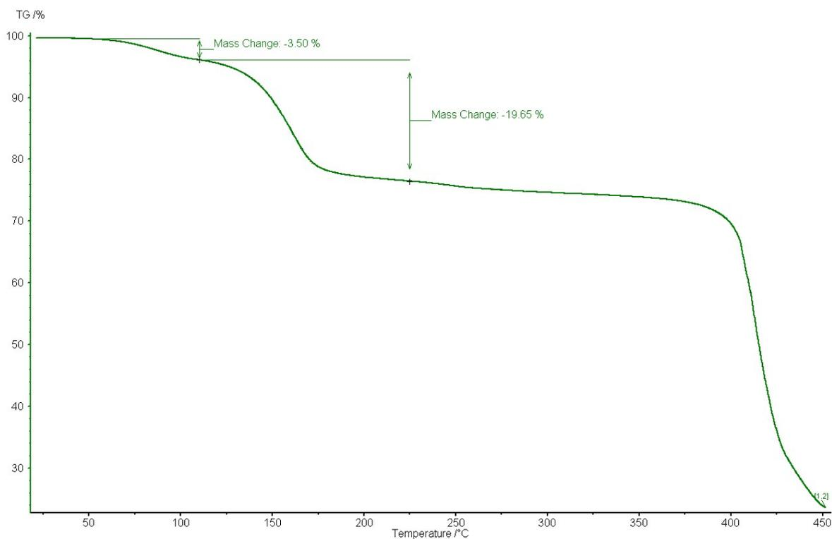
**Figure S2.1:** Thermogravimetric analysis of Compound 1. Overall mass loss (23.15%) corresponds to the loss of 10.93 water molecules, of which 1.65 water molecules are lost in the first step (25 to 110°C, 3.49%, non-coordinated water molecules) and 9.28 are lost in the second step (110 to 225°C, 19.65%, coordinated water molecules).
