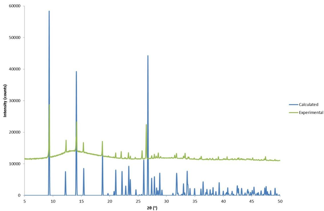
**Figure S1.4:** Calculated and experimental powder diffraction patterns for  $\text{Mn}(\text{HMeOip})_2$  (**4**).
