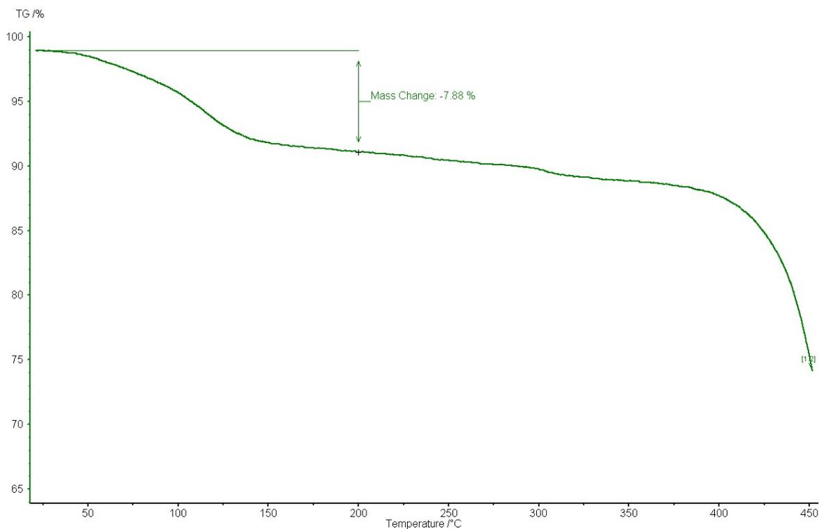
**Figure S2.3:** Thermogravimetric analysis of Compound **3**. The mass loss occurring over the temperature range 20°C to 200°C approximately corresponds to the loss of 6 water molecules (7.58%).
