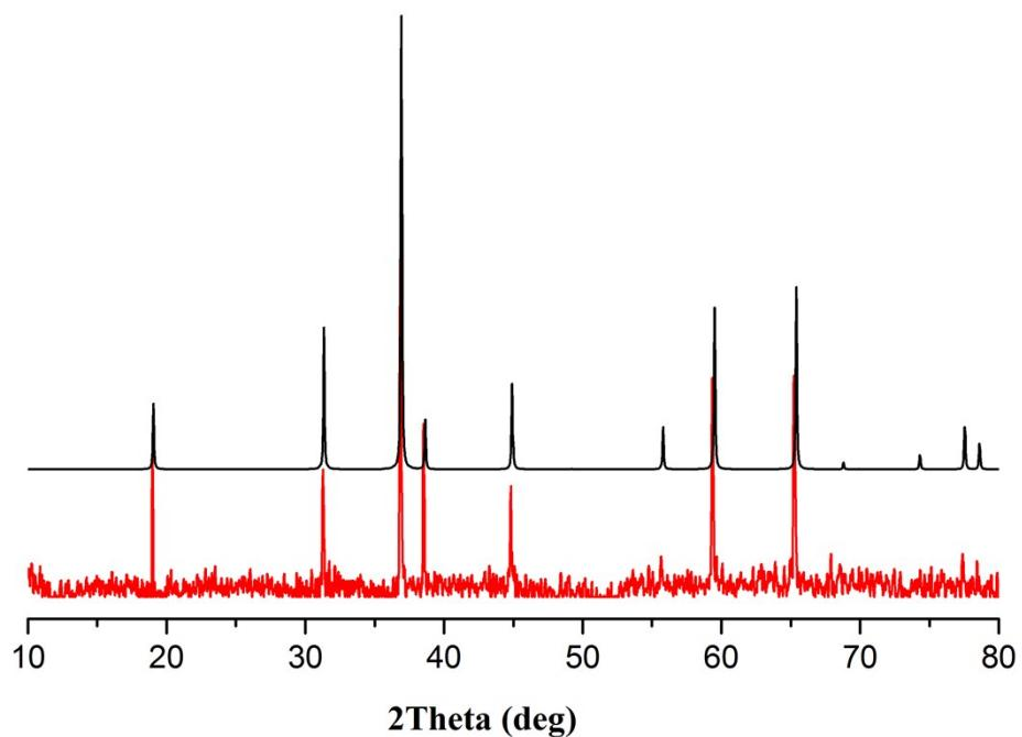
Figure S11 The simulated X-ray powder diffraction patterns of cubic  $\text{Co}_3\text{O}_4$  (black line, JCPDS card no. 43-1003) and the measured one (red line) of the residue after thermal decomposition of compound 1.
