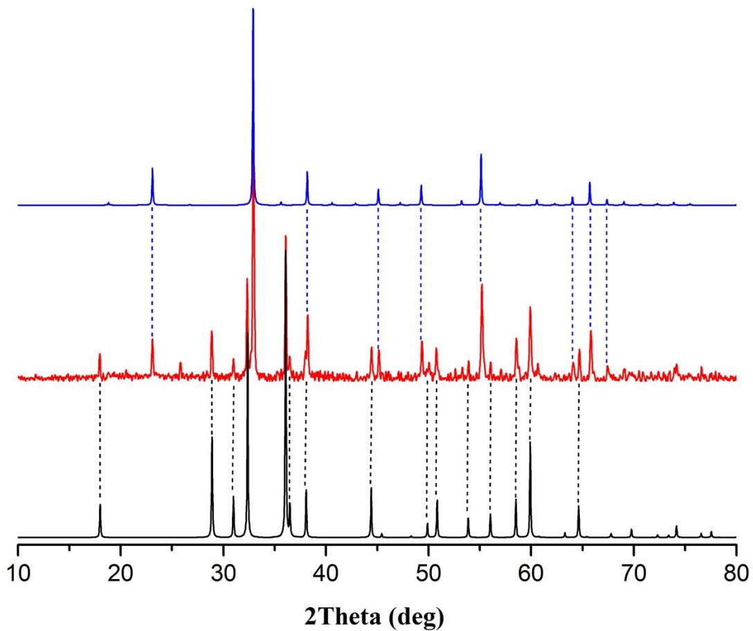
Figure S12 The simulated X-ray powder diffraction patterns of cubic  $\text{Mn}_2\text{O}_3$  (blue line, JCPDS card no. 41-1442), and tetragonal  $\text{Mn}_3\text{O}_4$  (black line, JCPDS card no. 24-0734), as well as the measured one (red line) of the residue after thermal decomposition of compound 2.
