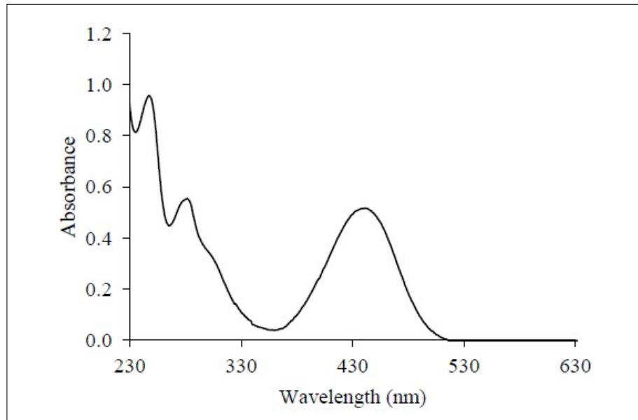
UV-Vis spectrum of a  $10^{-5}$  M solution of complex **1** in methanol.
