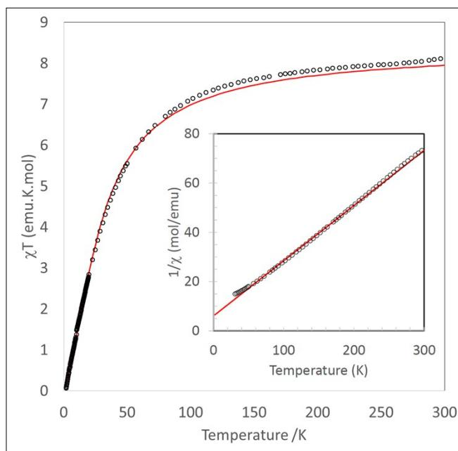
**Fig. 3.2** Temperature dependence of  $\chi T$  (per mole of dimer) for complex  $[\text{Mn}(\text{L9})\text{Cl}_2(\text{EtOH})]_2$  (**3**). The red line is the fit to the dimer model for two interacting  $S = 5/2$  ions.<sup>27</sup> Inset: Plot of  $1/\chi$  vs.  $T$  (per mole of  $\text{Mn}^{2+}$ ; the fit to the Curie Weiss law is shown as a red line).
