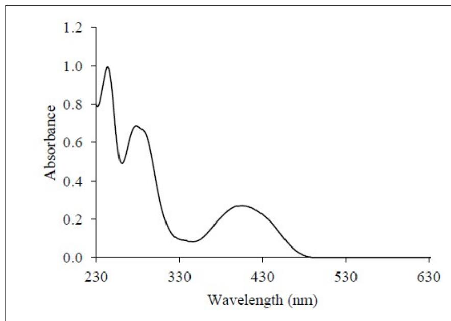
UV-Vis spectrum of a  $10^{-5}$  M solution of complex **2** in methanol.
