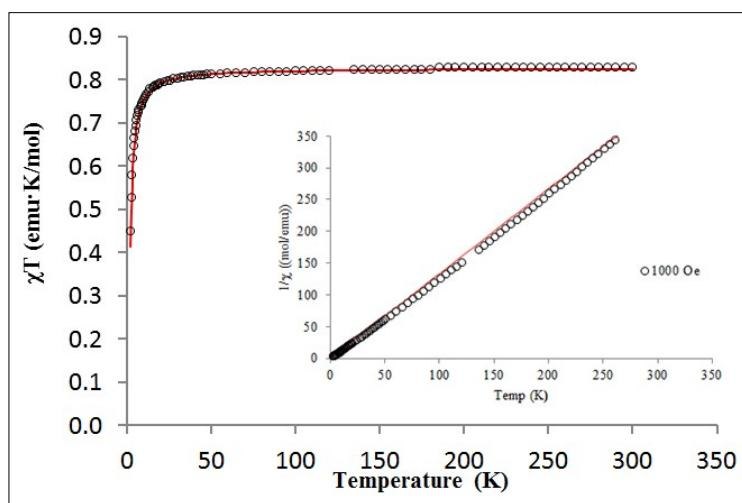
**Fig. 3.1**  $\chi T$  vs.  $T$  for  $[\text{Cu}(\text{L8})\text{sal}(\text{ClO}_4)_2]_2$  (**2**). The fit to the Bleaney-Bowers equation is shown as a red line.<sup>2</sup> Inset, plot of  $1/\chi$  vs.  $T$ ; the fit to the Curie Weiss law is shown as a red line.
