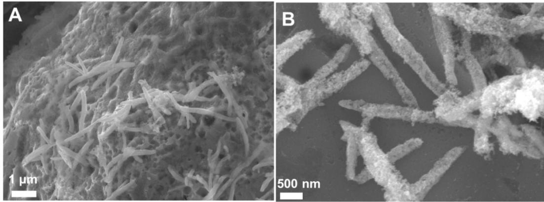
Figure S10, SEM images of the bare SnO<sub>2</sub> NA after cycling 100 cycles.
