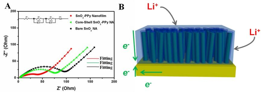
Figure S3, (A) Nyquist plots of bare  $\text{SnO}_2$  NA, core-shell  $\text{SnO}_2$ -PPy NA, and  $\text{SnO}_2$ -PPy nanofilm, (B) the schematic illustration of the  $\text{SnO}_2$ -PPy nanofilm in which the conducting polymer provides a flexible confinement for anchoring each nanorod and maintaining the whole structural integrity.
