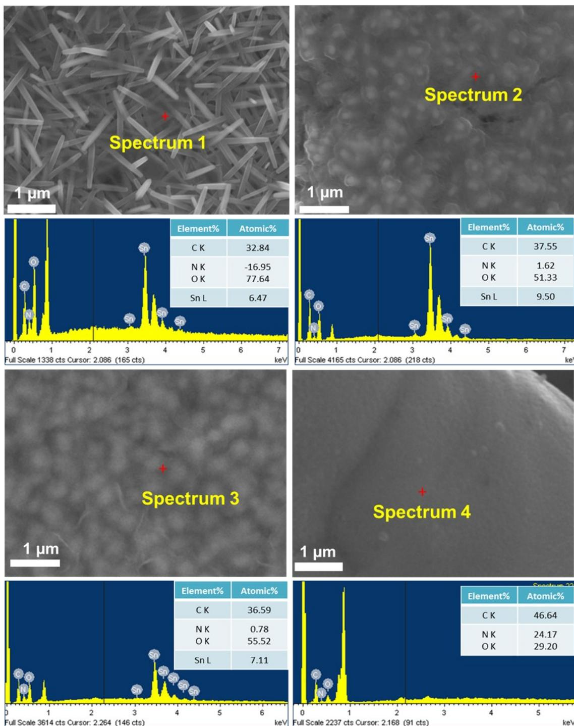
Figure S6, SEM images and the corresponding EDAX results of bare SnO<sub>2</sub> NA (A), core-shell SnO<sub>2</sub>-PPy NA (B), SnO<sub>2</sub>-PPy nanofilm (C) and bare PPy (D).
