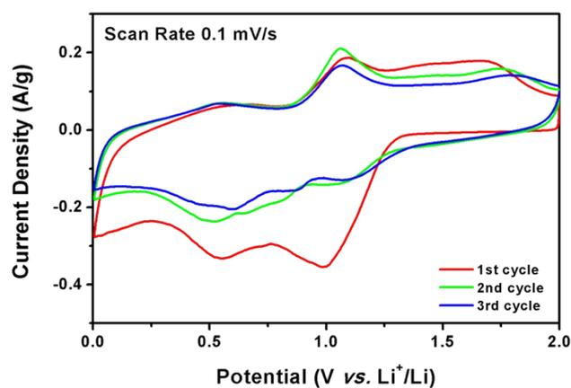
Figure S8, the CV curves of the SnO<sub>2</sub>-PPy nanofilm at scan rate of 0.1 mV/s.
