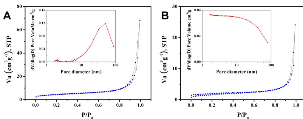
Figure S7, the nitrogen adsorption–desorption isotherm of bare SnO<sub>2</sub> nanorod (A) and the SnO<sub>2</sub>-PPy nanofilm (B).
