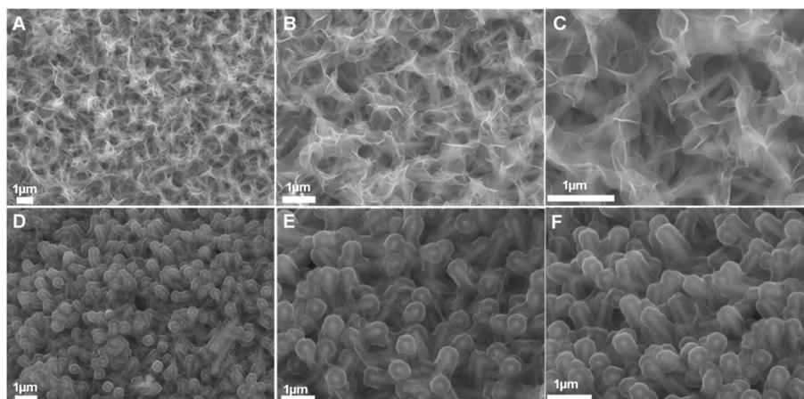
Figure S2, SEM image of the SnO<sub>2</sub>-PPy nanorod array with higher current density (A, B, C); the core-shell SnO<sub>2</sub>-PPy nanorod array (D, E, F).
