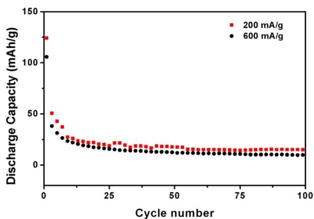
Figure S9, the cycle performance of bare PPy at current density of 200 and 600 mA/h/g at voltage window of 0.01-2 V.
