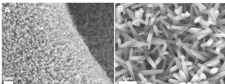
Figure S1, SEM image of the bare SnO<sub>2</sub> nanorod array
