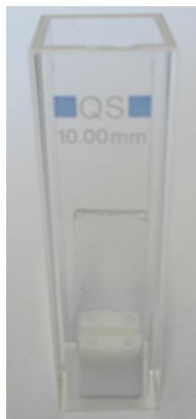
**Figure S1.** Set-up for UV-vis measurements of the quartz substrate bearing a porphyrin monolayer.
