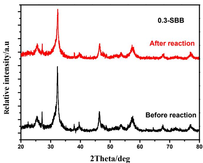
Fig. S1. XRD patterns of 0.3-SBB before and after photocatalytic reaction.
