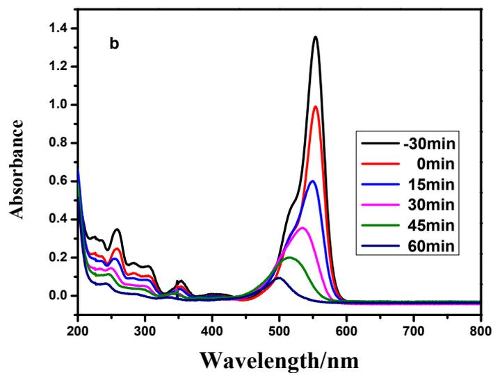
**Fig. S2.** UV-visible absorption spectral changes observed for the BiOBr/RhB (a) and 0.3-SBB/RhB (b) mixtures as a function of irradiation time under Xe arc lamp ( $\lambda > 420$  nm)
