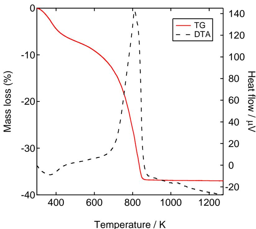
**Fig. S2** TG-DTA curves of TaOPc under flowing air. The heating rate was 10 K min<sup>-1</sup>.
