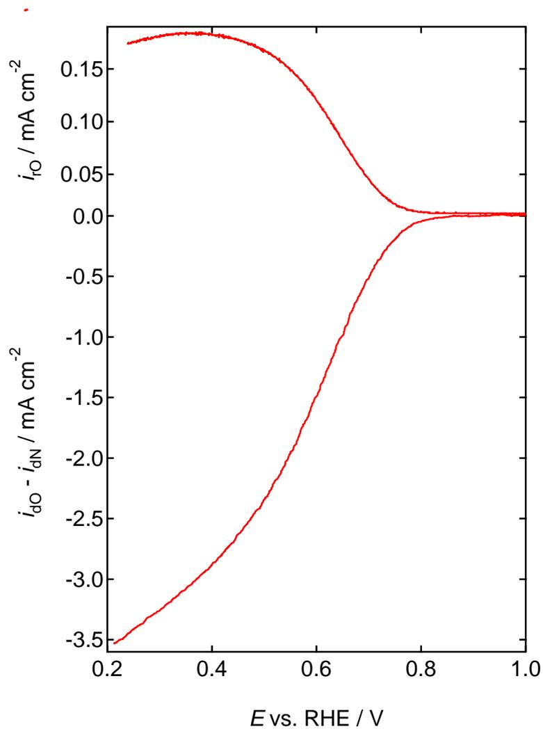
**Fig. S1** A RRDE voltammogram of TaO<sub>x</sub>-MWCNT after pyrolysis at 1173 K for 3 h under flowing a gas mixture of 2% H<sub>2</sub>, 0.5% O<sub>2</sub> and 97.5% N<sub>2</sub>. Scans were performed under N<sub>2</sub> and O<sub>2</sub> with a rotation speed of 1600 rpm at a scan rate of 5 mV s<sup>-1</sup> in the cathodic direction in 0.1 mol dm<sup>-3</sup> H<sub>2</sub>SO<sub>4</sub>. The TaO<sub>x</sub>-MWCNT loading was 1.6 mg cm<sup>-2</sup>.
