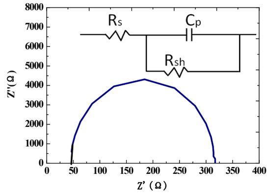
Fig S6. IS measurements(Nyquist plot) of CdS/Si NWs junctions in the dark. Inset shows the equivalent circuit for the same.
