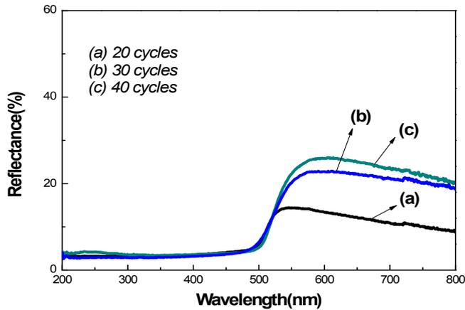
Fig.S3 The reflectance of CdS/SiNWA for different number of SILAR cycles
