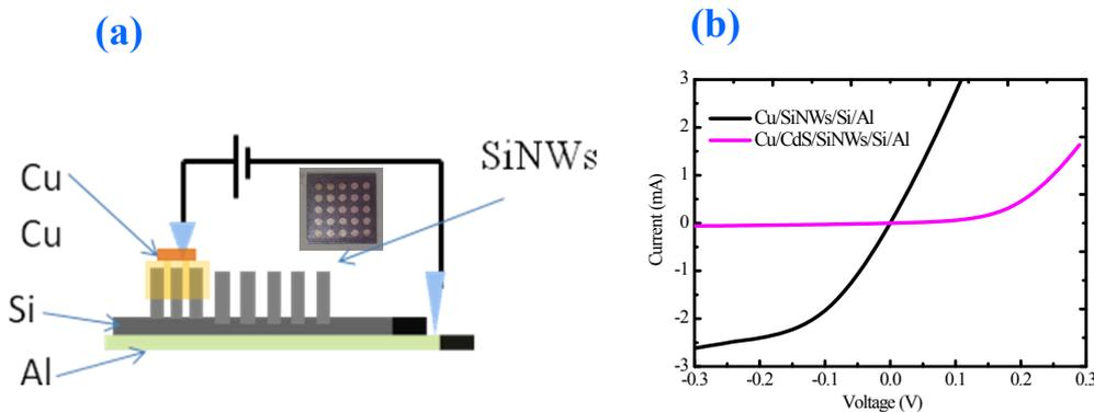
Fig.S5 (a) Schematic of the structure to measure the I-V across p-Si. The inset is photo of Al circle pats on Si NWs; (b) I-V characteristics of Cu/SiNWs/Si/Al and Cu/CdS/SiNWs/Si/Al
