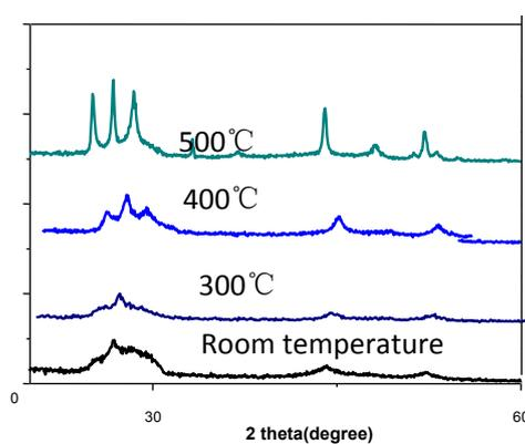
Fig.S1 The XRD patterns of different annealing temperature
