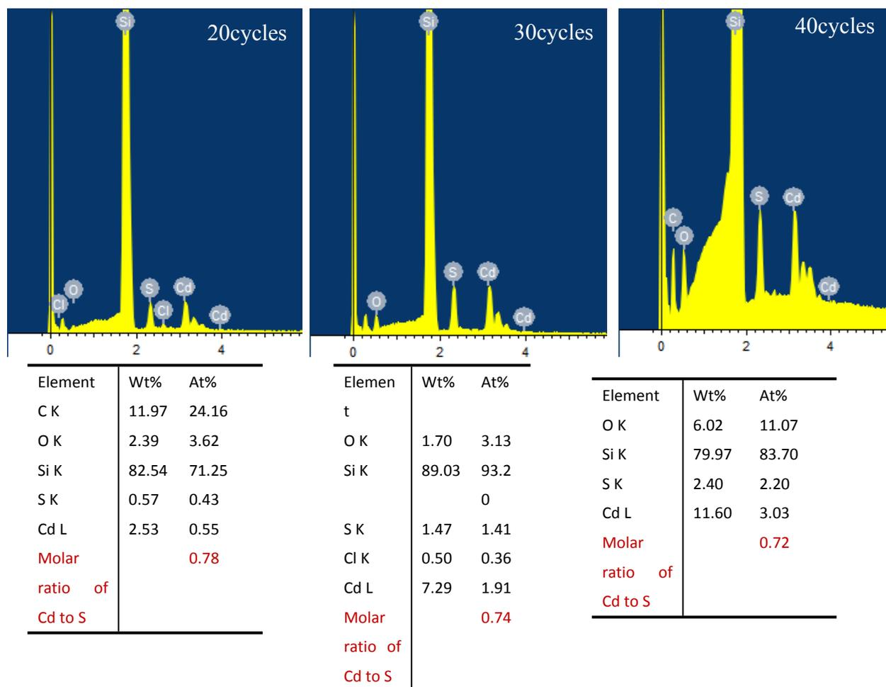
Fig.S2 The EDS spectra of CdS/SiNWA for different number of SILAR cycles
