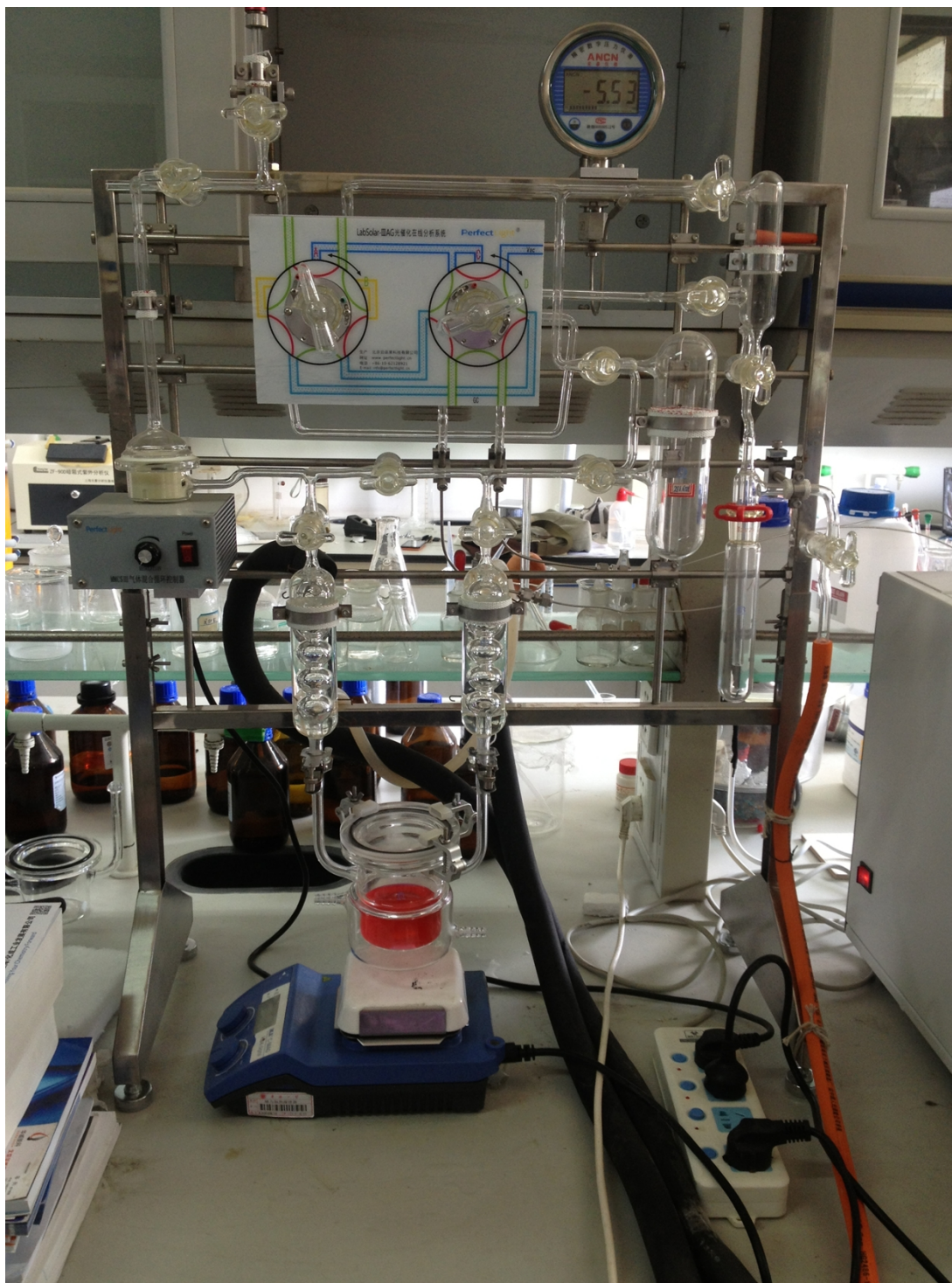
Fig. S1 Pyrex top-irradiation reaction vessel connected to a glass closed gas circulation system.
