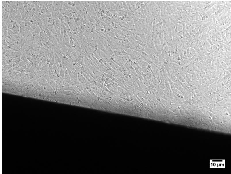
**Figure S8.** Bright-field microscope picture taken at the edge of a carbon coated filled nanocomposite sample. Cell confluence can be seen around the sample at the bottom of the well plate but not on the surface of the filled nanocomposites. This proves once more that even though the surface of filled nanocomposite samples doesn't allow cell proliferation, the samples do not show any toxic effect to fibroblasts.
