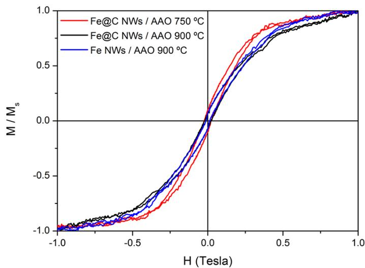
**Figure S3.** Normalized room-temperature hysteresis loops of nanocomposites filled with uncoated Fe NWs annealed at 900 °C and C-coated Fe NWs at 750 °C and 900 °C.
