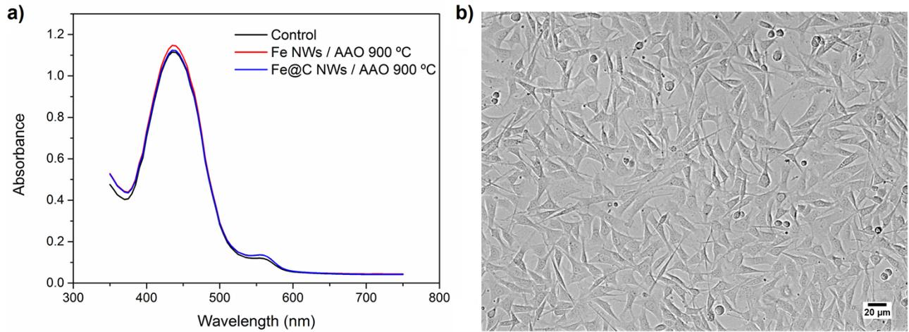
**Figure S6.** a) Absorption spectrum obtained from the WST-1 test for cells incubated in culture medium that was previously in contact with nanocomposites filled with Fe NWs and with C-coated Fe NWs. b) Fibroblast confluence in culture medium that was incubated previously with different AAO templates.
