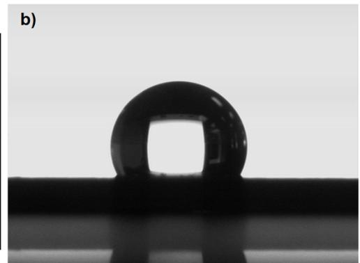
**Figure S5.** a) List of the measured surface contact angles obtained with different materials embedded in AAO. It was not possible to measure with the Young-Laplace method when the CVD temperature was 750 °C. b) Drop of culture medium on the surface of the nanocomposite.
