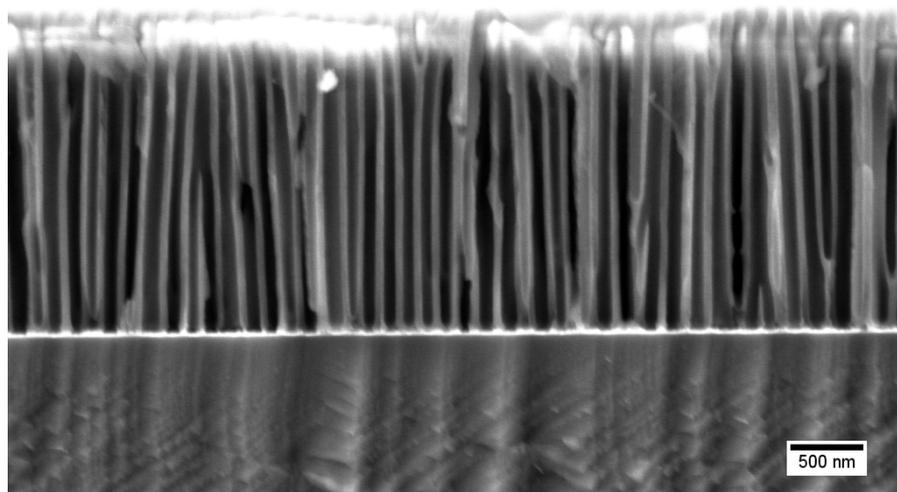
**Figure S1.** SEM image of the cross-section from the AAO template fabricated by anodization using oxalic acid at 60V. The template was etched with 5.5 wt% phosphoric acid to enlarge the pores and remove the barrier layer.
