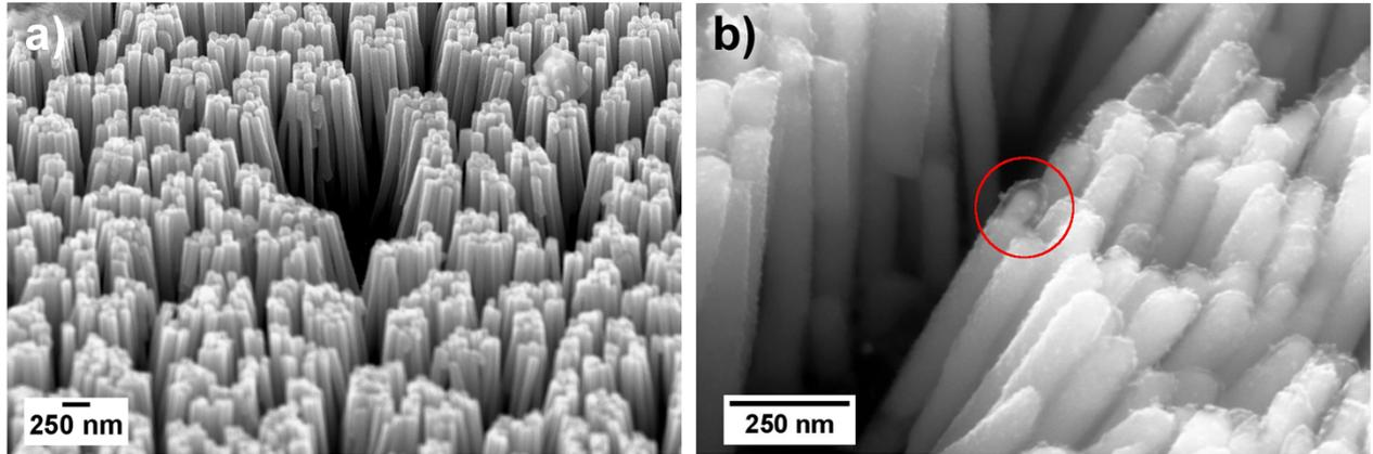
**Figure S2.** SEM images of a) uncoated and b) C-coated Fe NWs grown in AAO template. In b), the carbon coating of the core-multishell Fe@C NWs that was grown at 750 °C is highlighted. The AAO template was removed using a 10 wt% NaOH solution.
