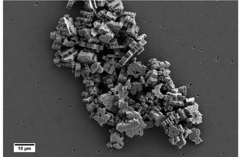
**Figure S4.** b) SEM image of the remaining AAO template after attempting its dissolution with the etchants listed on a) combined with high power tip sonication.
