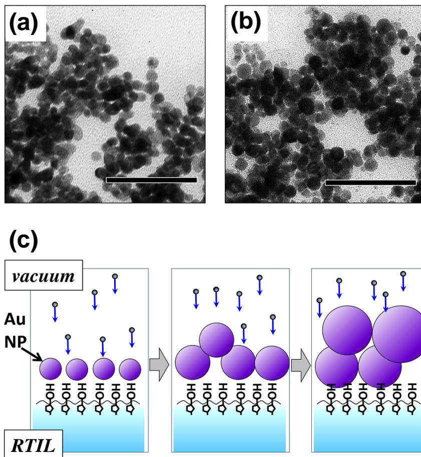
**Fig. S3** (a,b) TEM images of Au particles contained in multilayer particle films prepared by Au sputter deposition HyEMI-BF<sub>4</sub> for 600 (a) and 1200 s (b). The bars in pictures represent a length of 20 nm. Samples for TEM measurements were prepared by pulverizing multilayer particle films with sonication. (c) Schematic illustration of the multilayer film formation of Au particles along with collapse of monolayer by the crystal growth of individual particles on RTIL surface.
