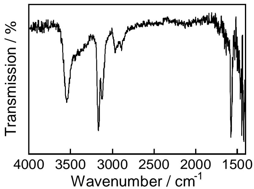
**Fig. S4** FT-IR spectrum of an Au monoparticle film immobilized on an Si substrate. The film was prepared by Au sputter deposition onto HyEMI-BF<sub>4</sub> for 300 s.
