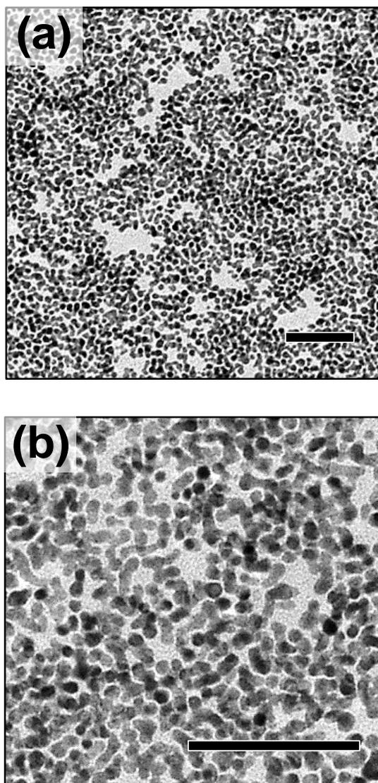
**Fig. S2** TEM images of Au monoparticle films prepared by sputter deposition of Au on HyEMI-BF4 for 30 s with a discharge current of 40 mA under an Ar pressure of 20 Pa. Panel b is a magnified image of panel a. The bars in pictures represent a length of 20 nm.
