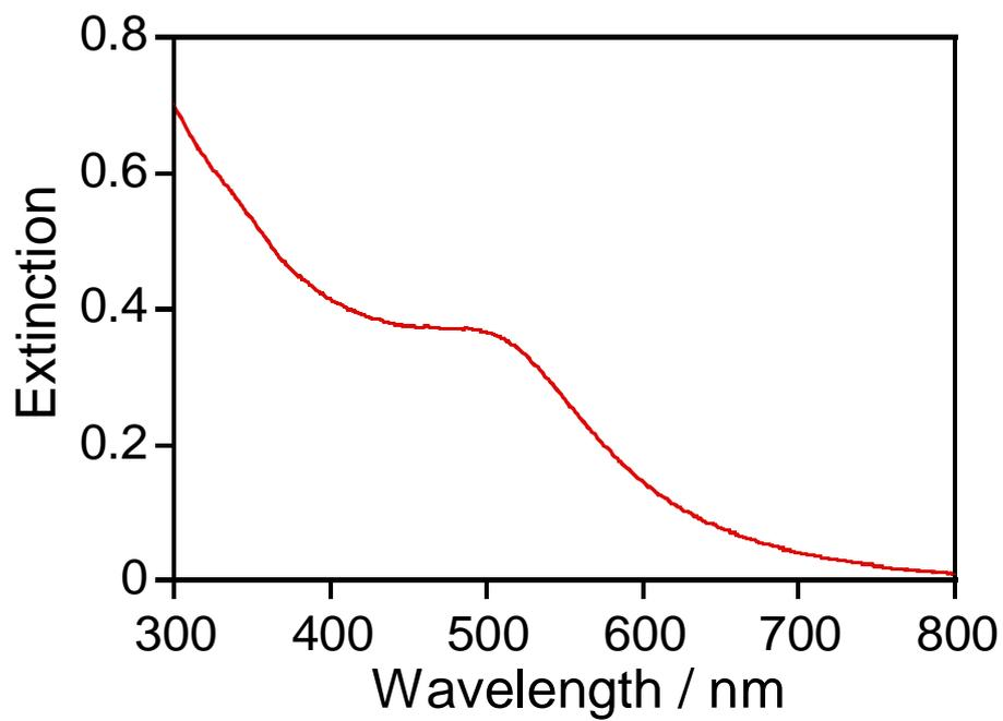
**Fig. S1** Extinction spectrum of Au nanoparticles uniformly dispersed in EMI-BF4. The particles were prepared by sputter deposition of Au on EMI-BF4 for 300 s with a discharge current of 10 mA under an Ar pressure of 20 Pa.
