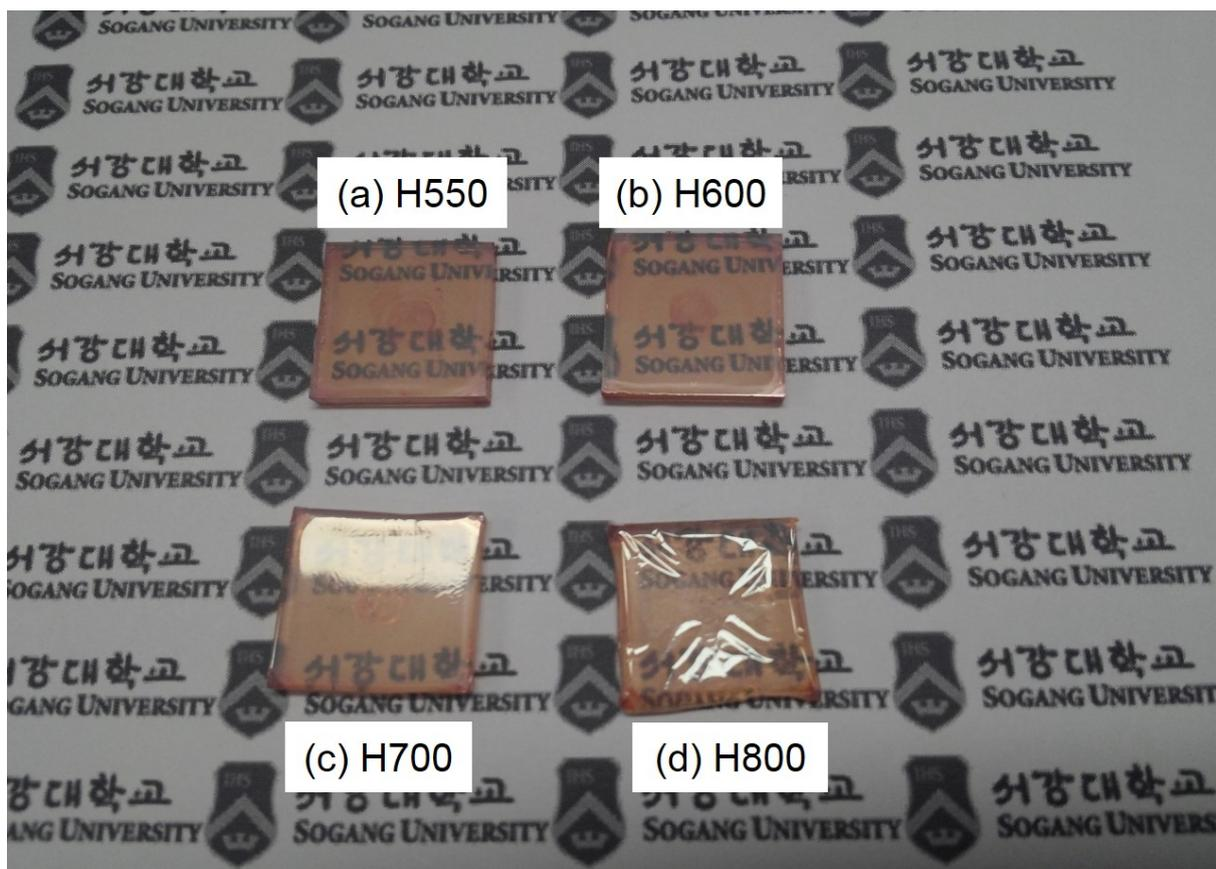
**Figure S2.** Digital pictures of H550, H600, H700 and H800 hematite thin films prepared by deposition and annealing (DA) method of 10 DA cycles.
