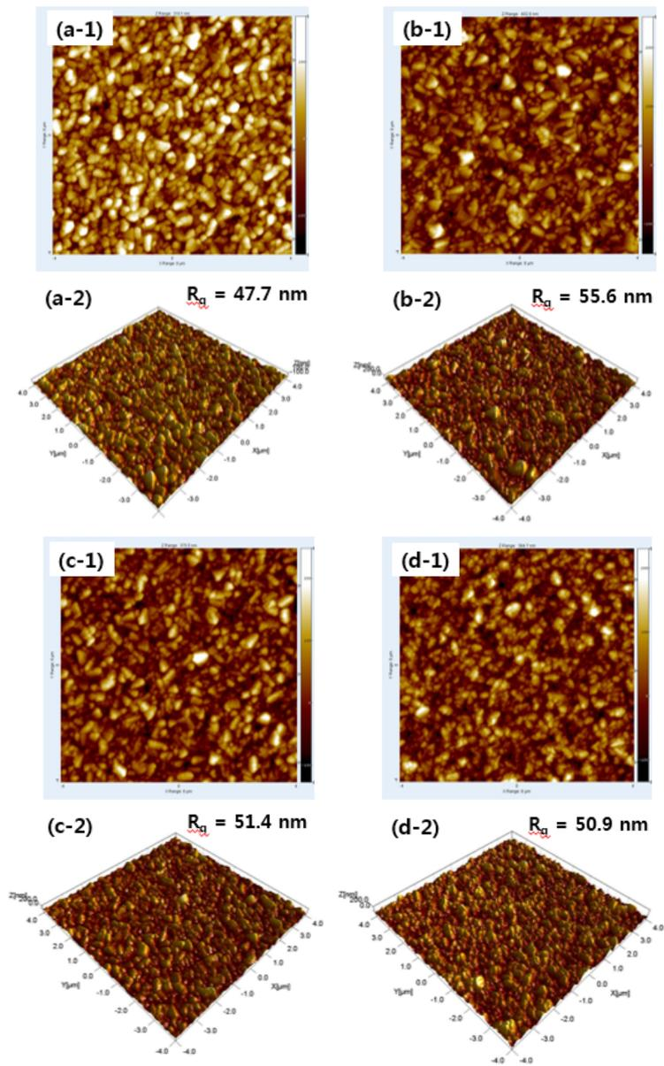
**Figure S5.** 2D and 3D atomic force microscopy scan images of 10DA hematite films H550 (a-1) and (a-2), H600 (b-1) and (b-2), H700 (c-1) and (c-2), H800 (e-1) and (e-2). (8x8  $\mu\text{m}$  image scale,  $R_q$  is root mean square roughness of surface)
