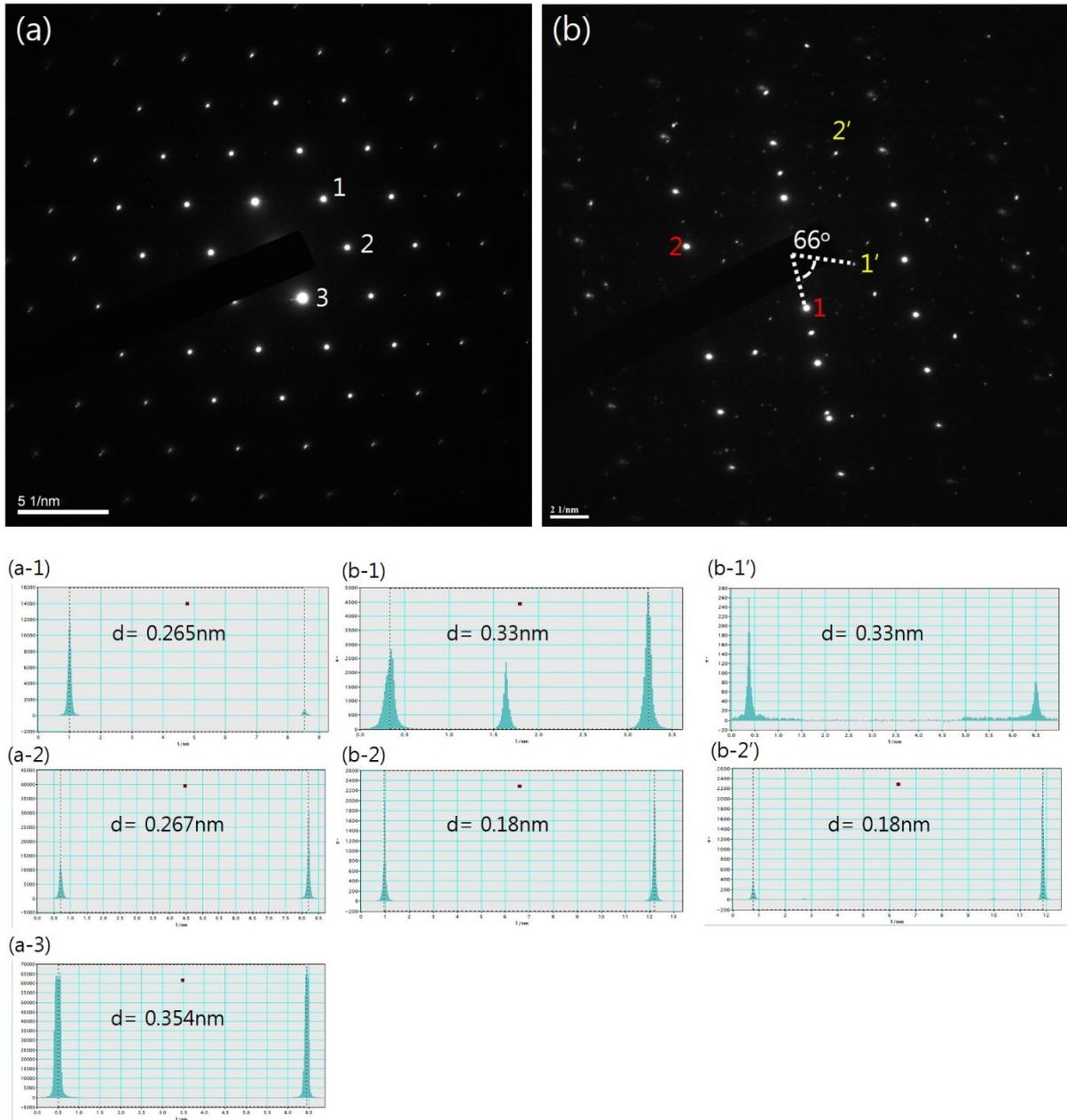
**Figure S8.** TEM SAED patterns of FTO substrate ( $\text{SnO}_2$ ) for (a) H700 and (b) H800 with 10 DA cycles. Spectrum line profile for spot 1 in H700 (a-1), spot 2 in H700 (a-2), spot 3 in H700 (a-3), spot 1 in H800 (b-1), spot 2 in H800 (b-2), tilted spot 1' in H800 (b-1') and spot 2' in H800 (b-2').
