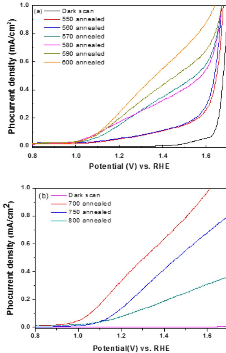
**Figure S9.** Photocurrent density curves of hematite thin films with 10 DA cycles at different annealing temperature. (a) 550 °C, 560 °C, 570 °C, 580 °C, 590 °C, 600 °C (b) 700 °C, 750 °C, 800 °C.
