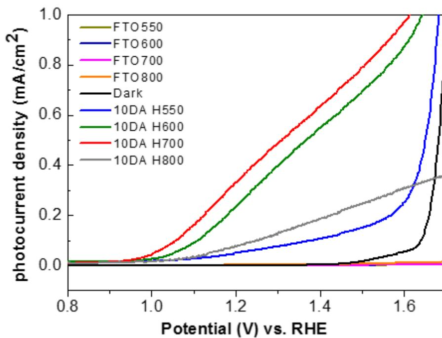
**Figure S12.** Photocurrent density curves of FTO550, FTO600, FTO700, FTO800, dark scan, H550, H600, H700, and H800 samples with 10 DA.
