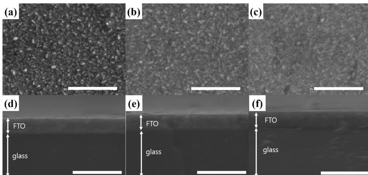
**Figure S3.** Top-view SEM images of H550 samples with (a) 20 DA (b) 30 DA and (c) 40 DA cycles (all scale bars are  $5\mu\text{m}$ ). Cross-sectional SEM images of H550 samples with (d) 20 DA (e) 30 DA and (f) 40 DA cycles (all scale bars are  $2\mu\text{m}$ ).
