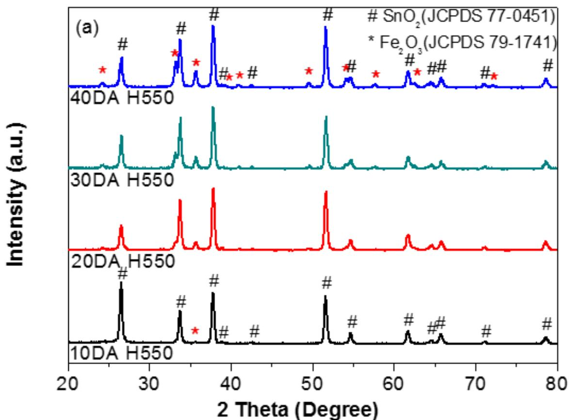
**Figure S6.** X-ray diffraction (XRD) patterns of H550 samples prepared with 10 DA, 20 DA, 30 DA, and 40 DA cycles (SnO<sub>2</sub> for JCPDS No. 77-0451 and a-Fe<sub>2</sub>O<sub>3</sub> for JCPDS No. 79-1741).
