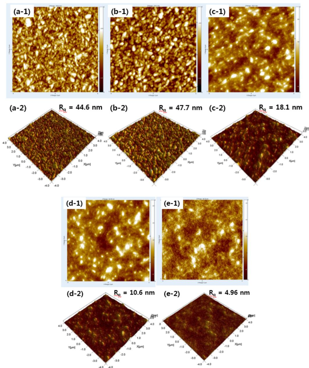
**Figure S4.** 2D and 3D atomic force microscopy scan images of bare FTO (a-1) and (a-2), H550 with 10 DA (b-1) and (b-2), H550 with 20 DA (c-1) and (c-2), H550 with 30 DA (d-1) and (d-2), H550 with 40 DA (e-1) and (e-2). (8x8  $\mu\text{m}$  image scale,  $R_q$  is root mean square roughness of surface).
