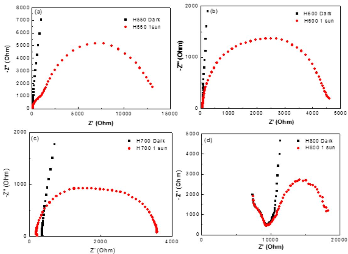
**Figure S10.** Nyquist plots of (a) H550, (b) H600, (c) H700, (d) H800 with 10 DA in dark condition and 1 sun illumination condition.
