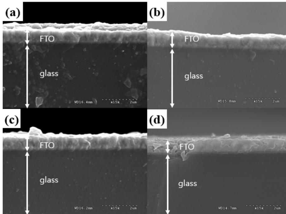
**Figure S1.** Cross-sectional SEM images of 10DA hematite films (a) H550 (b) H600 (c) H700 and (d) H800 (all scale bars are 2 $\mu$ m).
