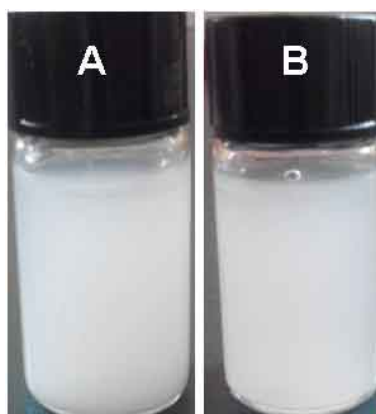
Fig. S4 Dispersibility of F127 modified HAp: 15\%\text{Tb}^{3+} (A) and HAp: 15\%\text{Eu}^{3+} (B) nanorods in pure water solution.
