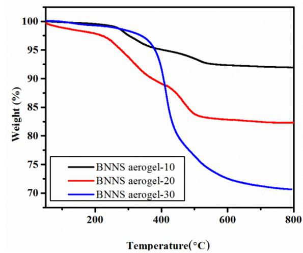
Figure S2. TGA of BNNS aerogels with different BDGE contents.
