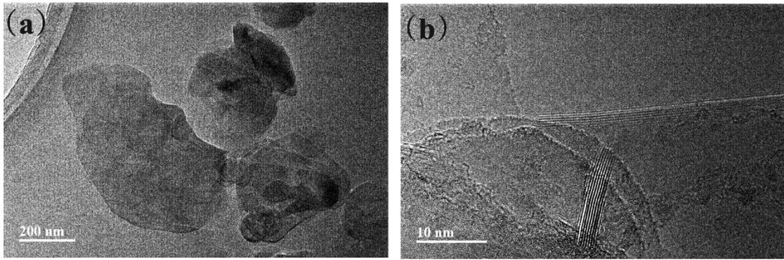
Figure S1. TEM micrographs of the BNNSs at low (a), and high (b) magnifications, respectively.
