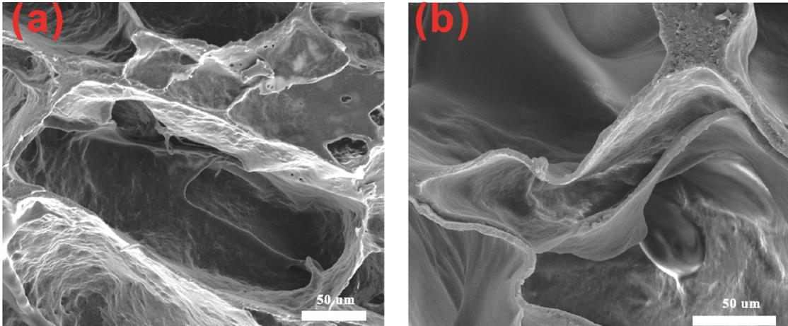
Figure S4. SEM micrographs of cellular structures of BNNS aerogel before (a), and after (b) irreversible compression.
