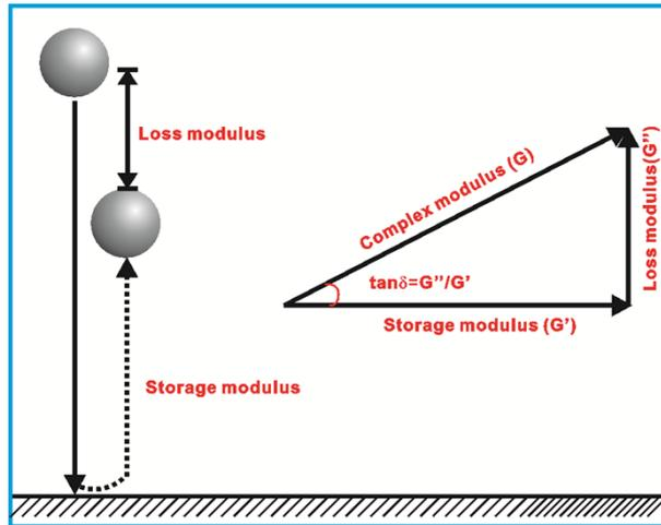
Figure S3. Schematic of viscoelastic property calculation procedure from stress-strain relation.
