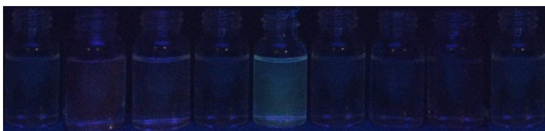
Figure S11: Colour change induced upon addition of (excess equivalents of perchlorate salts) different metal ions to Z-DPYDPE (in CH 3 CN) under UV lamp: From left to right: (1) no metal ion, (2) Zn 2+ , (3) Cu 2+ , (4) Fe 2+ , (5) Hg 2+ , (6) Ni 2+ , (7) Co 2+ , (8) Cd 2+ , (9) Mn 2+
