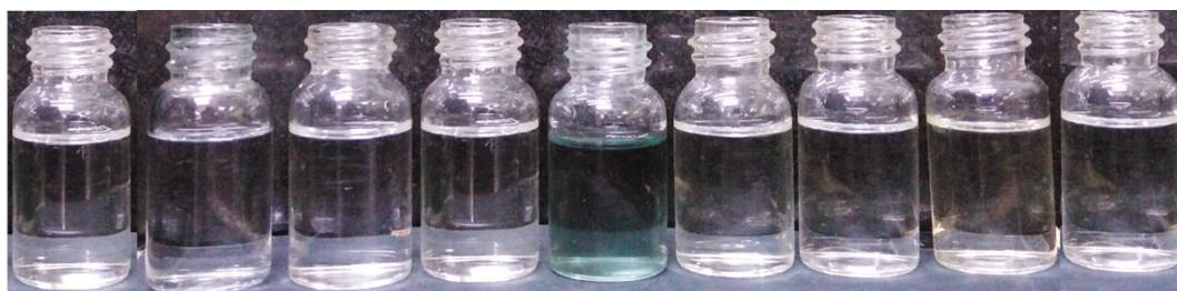
Figure S10: Colour change induced upon addition of (excess equivalents of perchlorate salts) different metal ions to Z-DPYDPE (in \text{CH}_3\text{CN} ) under daylight: From left to right: (1) no metal ion, (2) \text{Zn}^{2+} , (3) \text{Cu}^{2+} , (4) \text{Fe}^{2+} , (5) \text{Hg}^{2+} , (6) \text{Ni}^{2+} , (7) \text{Co}^{2+} , (8) \text{Cd}^{2+} , (9) \text{Mn}^{2+}
