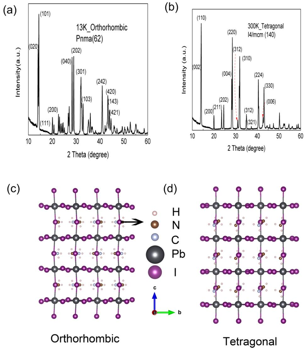
Fig.S3 (a) and (b): XRD patterns of MAPbI<sub>3</sub> perovskite at 13 and 300 K, respectively; (c) and (d): crystal structures of the tetragonal and orthorhombic MAPbI<sub>3</sub> perovskite.
