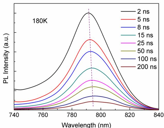
Fig. S2 TRPL spectra of the MAPbI<sub>3</sub> measured at (a) 300K, (b) 260K, (c) 220K and (d) 180K.
