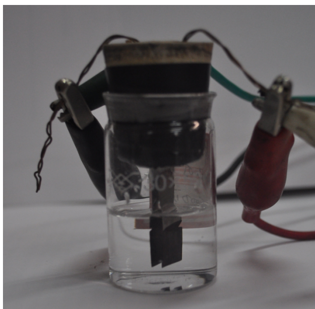
Fig. S1 a photograph of the fabricated supercapacitor, and the distance between two electrodes was about 2 mm.
