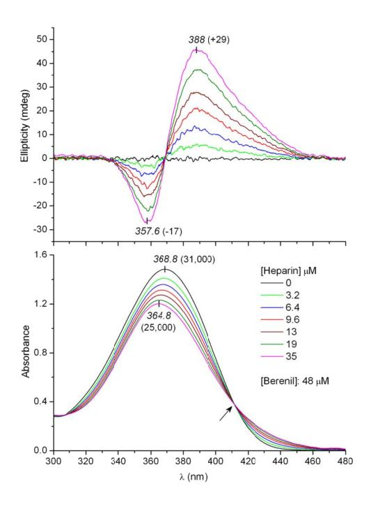
Induced CD and absorption spectra of 48  $\mu$ M berenil at increasing concentrations of heparin in deionized water (100 mM NaCl, 25 °C). Molar absorption ( $\epsilon$ ) and circular dichroic absorption cofficients ( $\pm\Delta\epsilon$ )calculated by using the concentration of berenil in the sample solution are shown in parentheses. Arrow denotes an isosbestic point at 411 nm.
