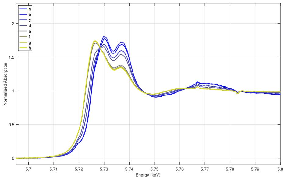
Figure 1: Normalised Ce  $L_{III}$  edge absorption spectra recorded during reduction of  $Ce_{0.9}Hf_{0.1}O_{2-\delta}$  powder diluted with BN by heating with a rate of  $50 Kmin^{-1}$  from RT (a) to 1073 K (f,g,h) in a flow of helium. Kapton windows were used.
