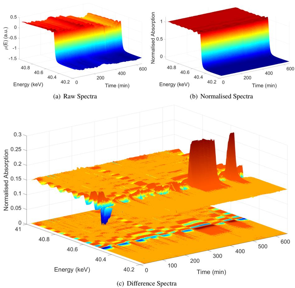
Figure 3: (a) Cerium K edge X-ray absorption spectra, (b) after normalization and (c) difference spectra obtained by subtraction of a spectrum recorded at 1073 K after the first reduction by flushing the reactor with argon at 1773 K.
