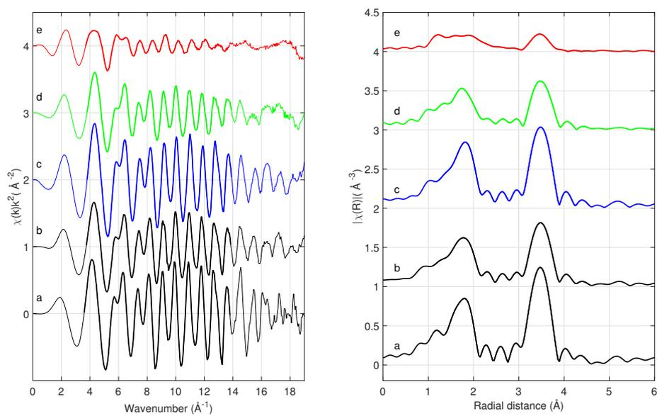
Figure 4: Extended X-ray absorption fine structure (EXAFS) of a)  $\text{CeO}_2$  (as prepared) b)  $\text{CeO}_{1.93}$  (reduced Ar) c)  $\text{Ce}_{0.9}\text{Hf}_{0.1}\text{O}_2$  (as prepared) d)  $\text{Ce}_{0.9}\text{Hf}_{0.1}\text{O}_{1.92}$  and e)  $\text{Ce}_{0.9}\text{Hf}_{0.1}\text{O}_{1.55}$  (reduced  $\text{H}_2$ ) recorded at RT. The bold lines indicate the data range used for Fourier-transformation of  $\chi(k)$  to obtain the pseudo-radial distribution functions  $\chi(R)$ .
