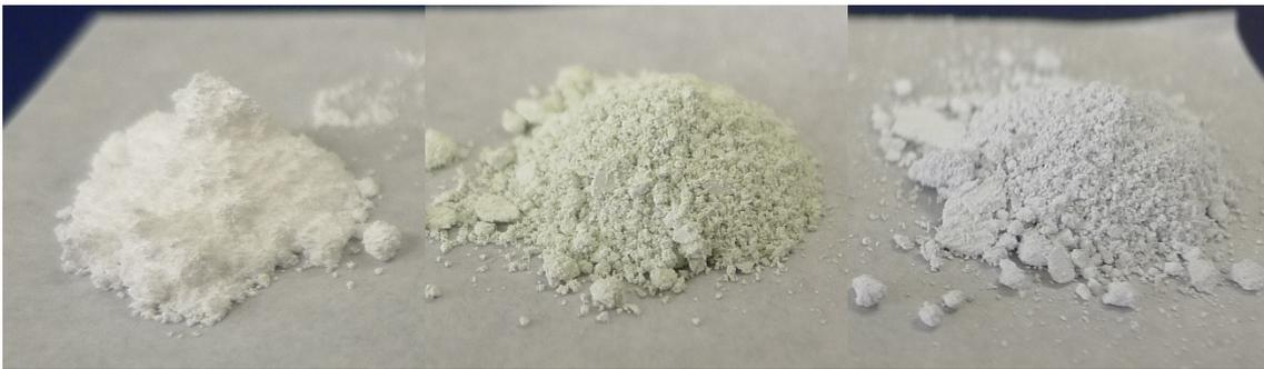
**Figure S2.** Photographs of decahedral TiO<sub>2</sub> nanoparticles. From left: bare decahedral TiO<sub>2</sub>, after 40 min plasma treatment, and after alkaline treatment.
