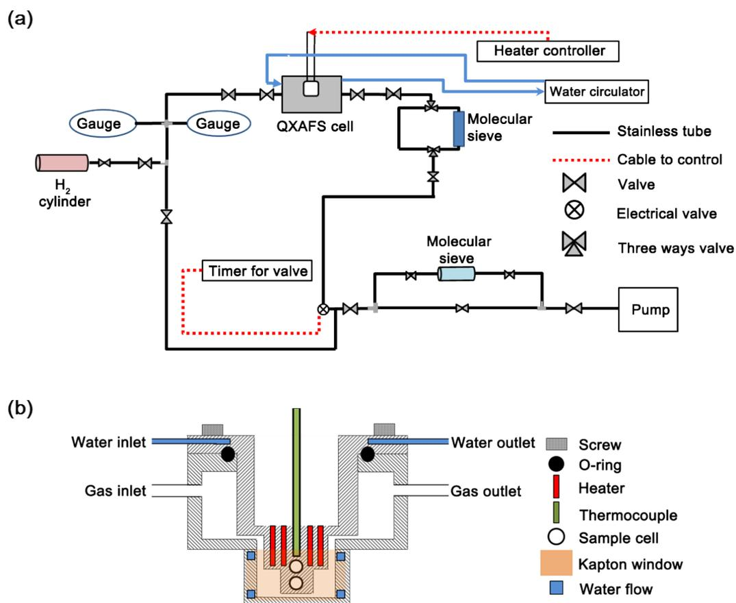
**Fig. S1** (a) Setup for in situ QXAFS measurements and (b) side view of the in situ QXAFS cell.
