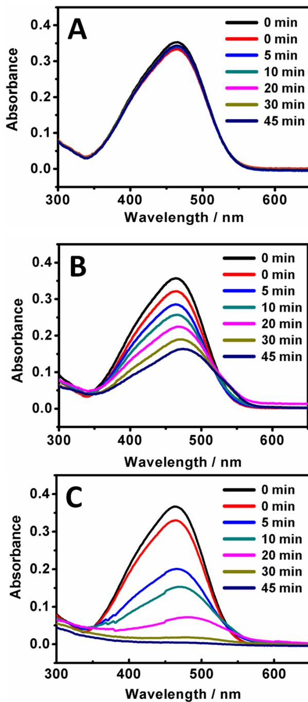
**Fig. S7** The real-time absorption spectra of MO molecules measured during the photocatalytic performances. A): The result obtained from a blank experiment, wherein no photocatalysts are involved. B) and C): The employed photocatalysts are the near-spherical (B) and fibrous (C) Ag/AgCl structures. The black and red curves marked as 0 minute are the absorption spectra detected from the original MO solution before (black) and after (red) the dark adsorption experiments, respectively.
