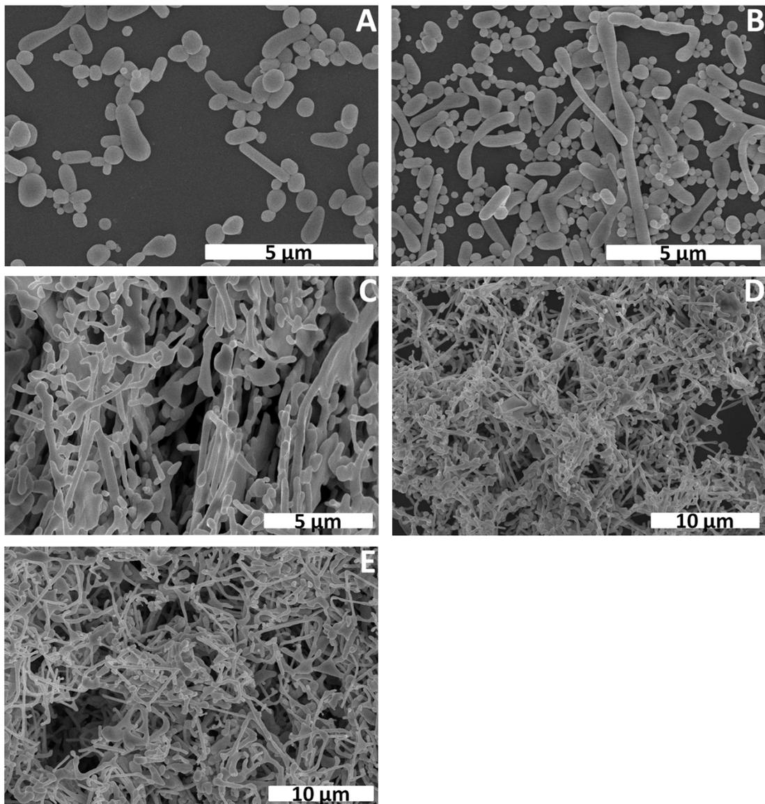
**Fig. S2** The SEM images of the as-manufactured structures as a function of the stirring time, wherein a CTAC dispersion of a concentration of  $4 \times 10^{-2}$  M is used as the host solution. The stirring time is 1, 12, 24, 48 and 72 hours for panel A, B, C, D and E, respectively.
