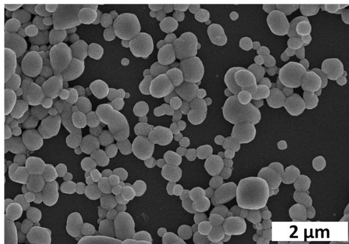
**Fig. S3** The SEM image of the originally produced near-spherical Ag/AgCl structures, which were treated by stirring in pure Milli-Q water under ambient conditions for 36 hours.
