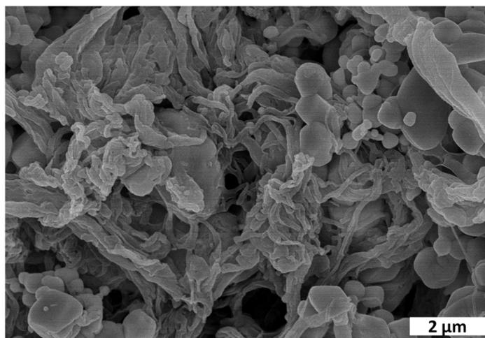
**Fig. S5** The SEM image of the originally produced near-spherical Ag/AgCl structures, which were treated by stirring in a CTAC aqueous solution of a high-concentration ( $4 \times 10^{-2} \text{ mol L}^{-1}$ ) under ambient conditions for 36 hours.
