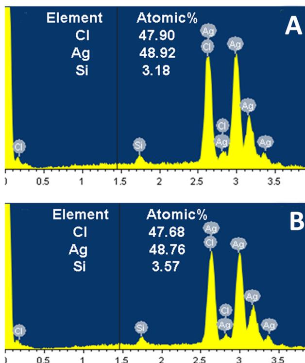
**Fig. S1** EDX elemental analysis of the as-fabricated near-spherical (A) and 1D (B) structures. The semiquantitative elemental analysis results for each sample are listed in the corresponding panels. Besides those attributed to Ag and Cl elements, EDX signals ascribing to Si element could also be detected, since Si plates were used as the solid support for the measurements.
