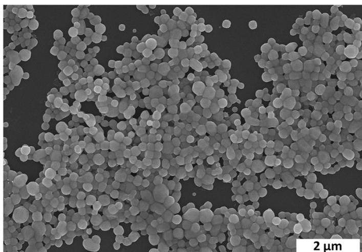
**Fig. S6** The SEM image of the samples fabricated by dropping an aqueous solution of  $\text{AgNO}_3$  into a low-concentration CTAC aqueous solution ( $4 \times 10^{-3} \text{ mol L}^{-1}$ ), wherein the as-produced dispersion was stirred under ambient conditions for 36 hours.
