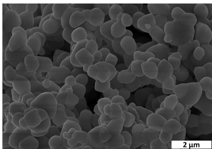
**Fig. S4** The SEM image of the originally produced near-spherical Ag/AgCl structures, which were treated by stirring in a CTAC aqueous solution of a low-concentration ( $4 \times 10^{-3} \text{ mol L}^{-1}$ ) under ambient conditions for 36 hours.
