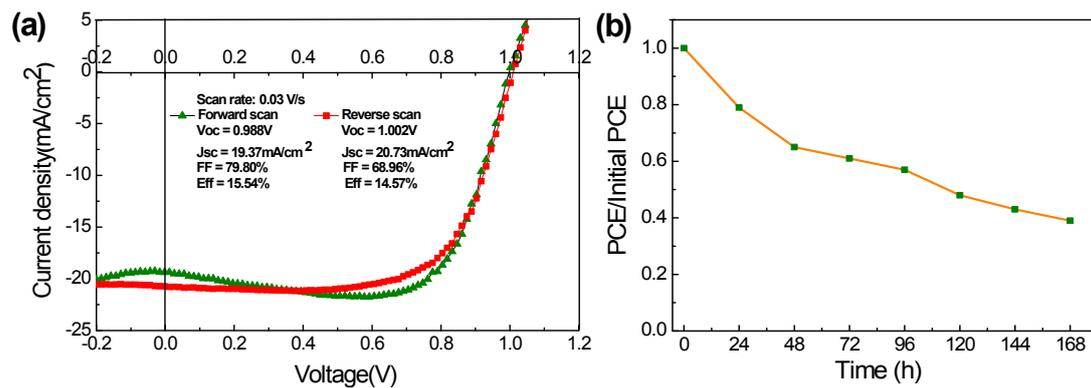
**Figure S4.** The  $J$ - $V$  hysteresis analyze (a) and stability as a function of time (b) of the perovskite solar cell.
