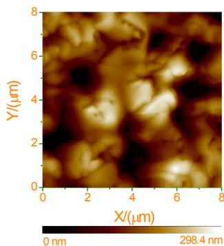
**Figure S2.** AFM image of the same perovskite /c-TiO<sub>2</sub> sample characterized in **Figure 3**.
