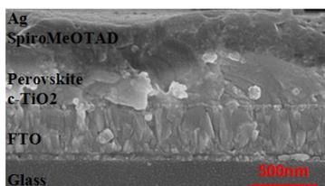
**Figure S3.** Cross-sectional SEM image of the device with a structure of Glass/FTO/c-TiO<sub>2</sub>/Perovskite/SpiroMeOTAD/Ag
