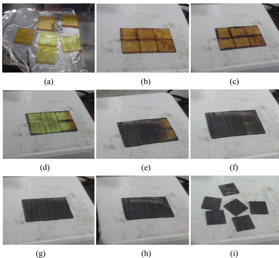
**Figure S1.** Optical images of the perovskite film heated at different stage, 0 min (a), 5 min (b), 15 min (c), 55 min (d), 65min (e), 75 min (f), 85 min (g), 95 min (h), 105 min (i), respectively.
