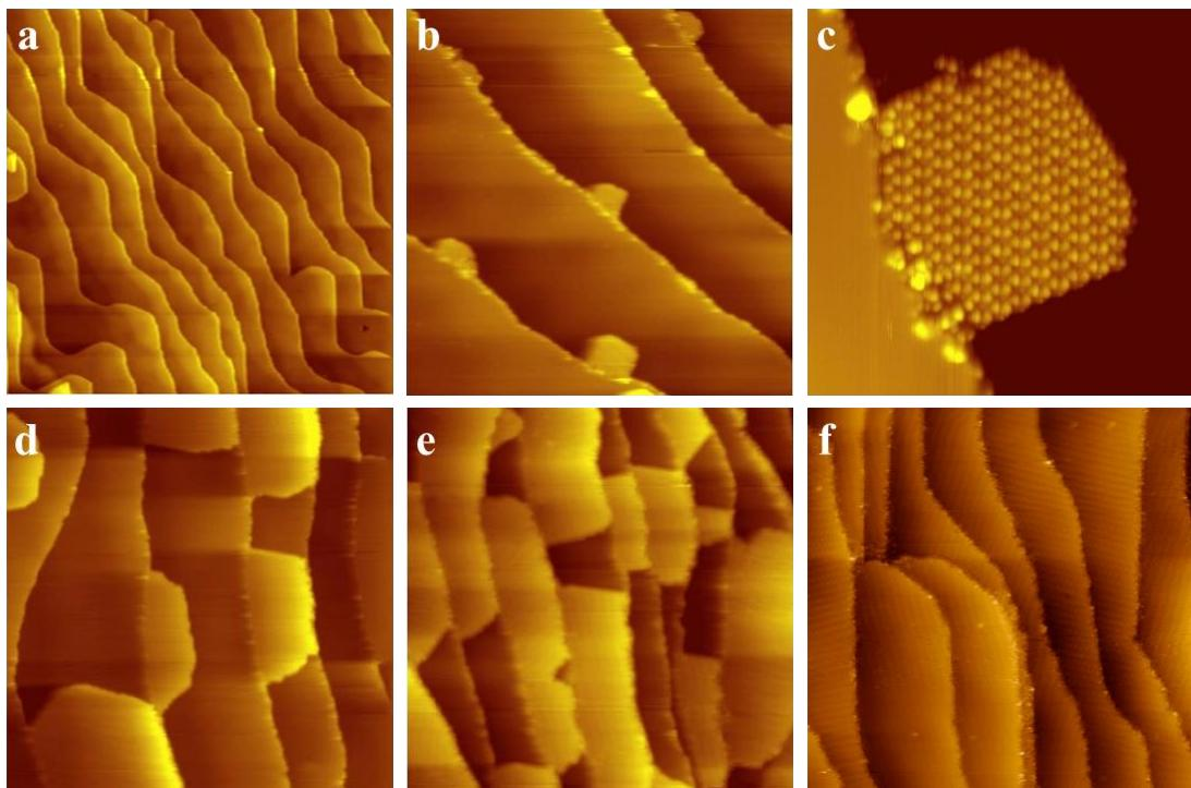
SI. 1 Anisotropic diffusion of homochiral domains of rubrene monomers at different coverage. (a) Flat and well-ordered Bi(111) substrate, 550 nm × 550 nm, +5.7V. (b) Homochiral domains at 0.1ML, 176 nm × 176 nm, +3.9V. (c) High-resolution images of a R- homochiral island, 30 nm × 30 nm, +3.1V. (d) Homochiral domains at 0.4ML, 200 nm × 200 nm, +4.2V. (e) Homochiral domains at 0.7ML, 180nm × 180nm, +3.9V (f) Homochiral domains at 1ML, 200 nm × 200 nm, +4.0V.
