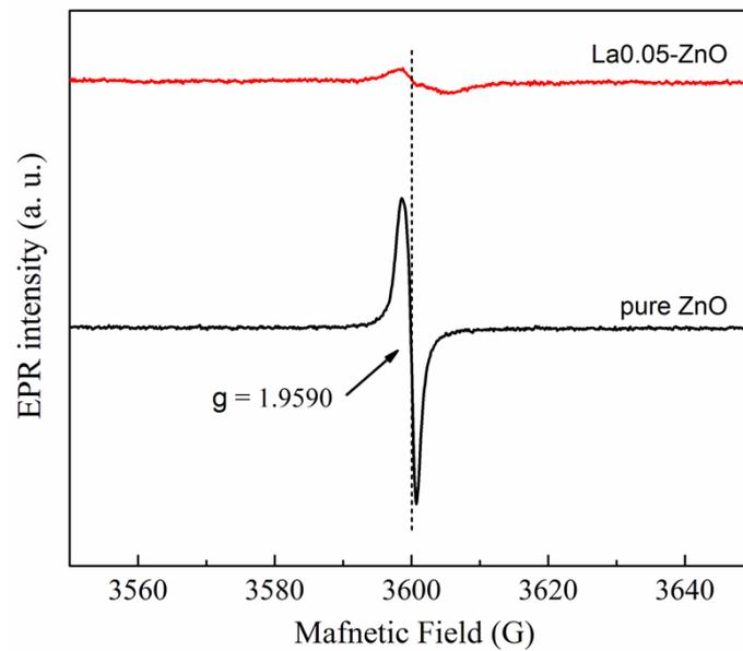
**Figure S1** EPR spectra measured at room temperature from pure ZnO and La0.05-ZnO.
