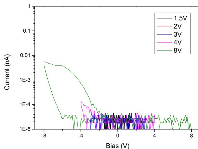
**Figure S2.** Locally acquired  $I-V$  curves of resistive switching behavior for the as-grown BTO film cooled at  $100\text{Torr}$  oxygen pressure.
