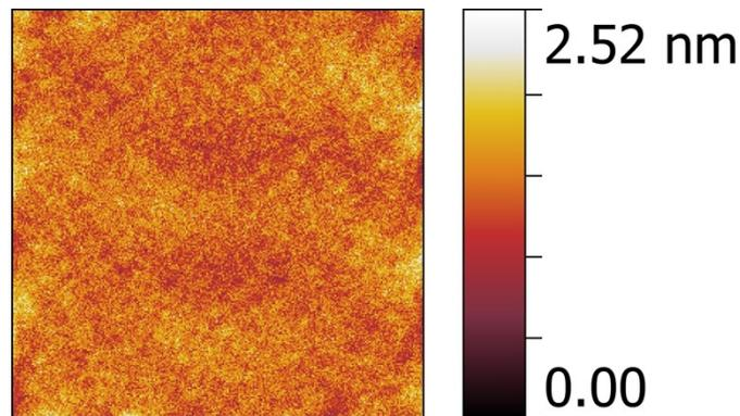
**Figure S1.** Topography image of BTO film cooled at  $50\mu\text{Torr}$  with a root-mean-square surface roughness of  $0.25\text{nm}$
