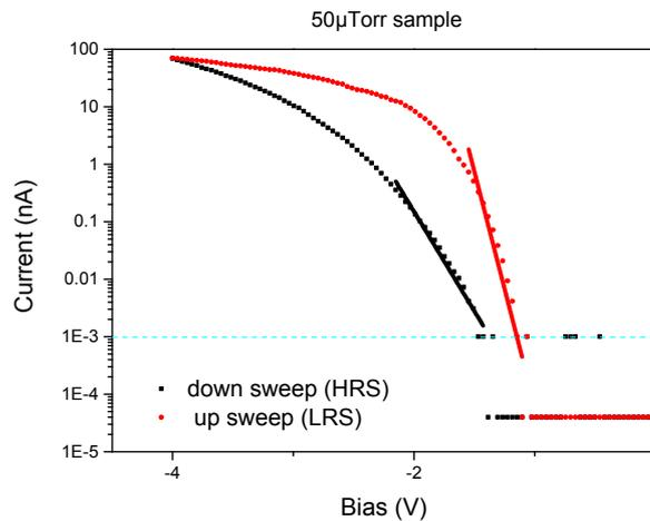
**Figure S3.** Linear fitting of the log I-V curve in the low voltage region for 50 $\mu$ Torr sample
